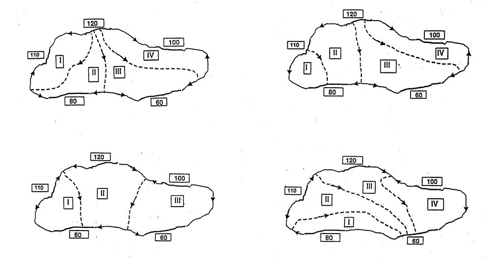
Figure 2: Four possible flow configurations, (A) One inlet and four outlets; (B) Two inlets and 3 outlets; (C) Three inlets and two outlets, and, (D) Four inlets and one outlet
