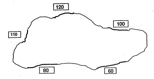
Figure 1: A flow domain with 5 boundary segments on which potentials are prescribed
