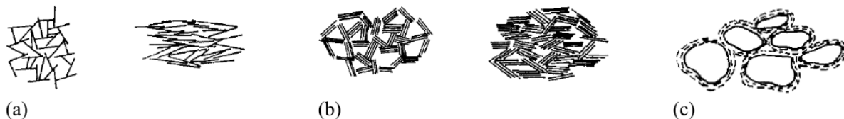
Figure 4-1. Schematic representation of elementary particle arrangements: (a) individual clay lamella or platelet, (b) clay platelet group interaction, and (c) clothed silt or sand particle interaction (Collins and McGown, 1974).
