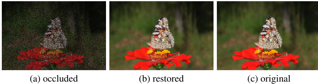
Figure 4.7: Pixel interpolation. (a) input image. (b) restored image for masking half pixels in (a).
