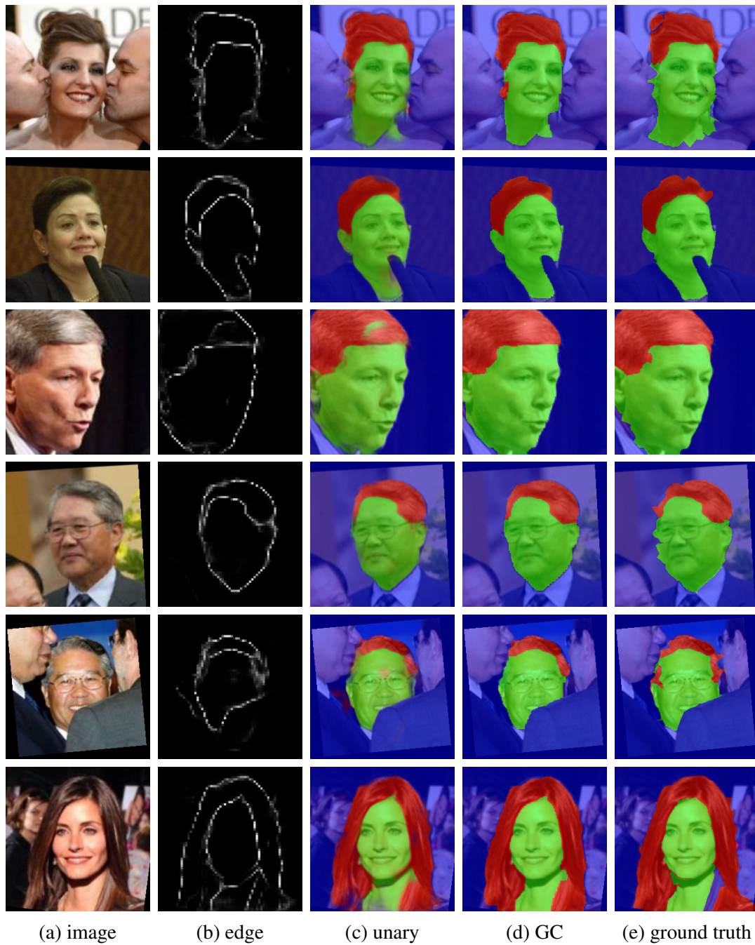
Figure 3.8: Face labeling results and semantic edge maps from LFW-PL dataset. (a) test images; (b) edge term output; (c) unary term output; (d) labeling result by GraphCut inference, denoted as GC; (e) ground truth. Best viewed in colors.
