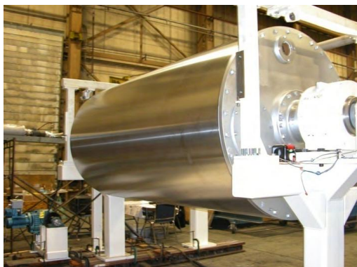
Figure 20. Photo of gas-fired dryer (Chudnovsky 2011)
