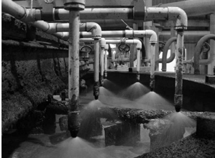
Figure 15. Surfactant spray deinking in a mill trial (Deng and Zhu 2004)
