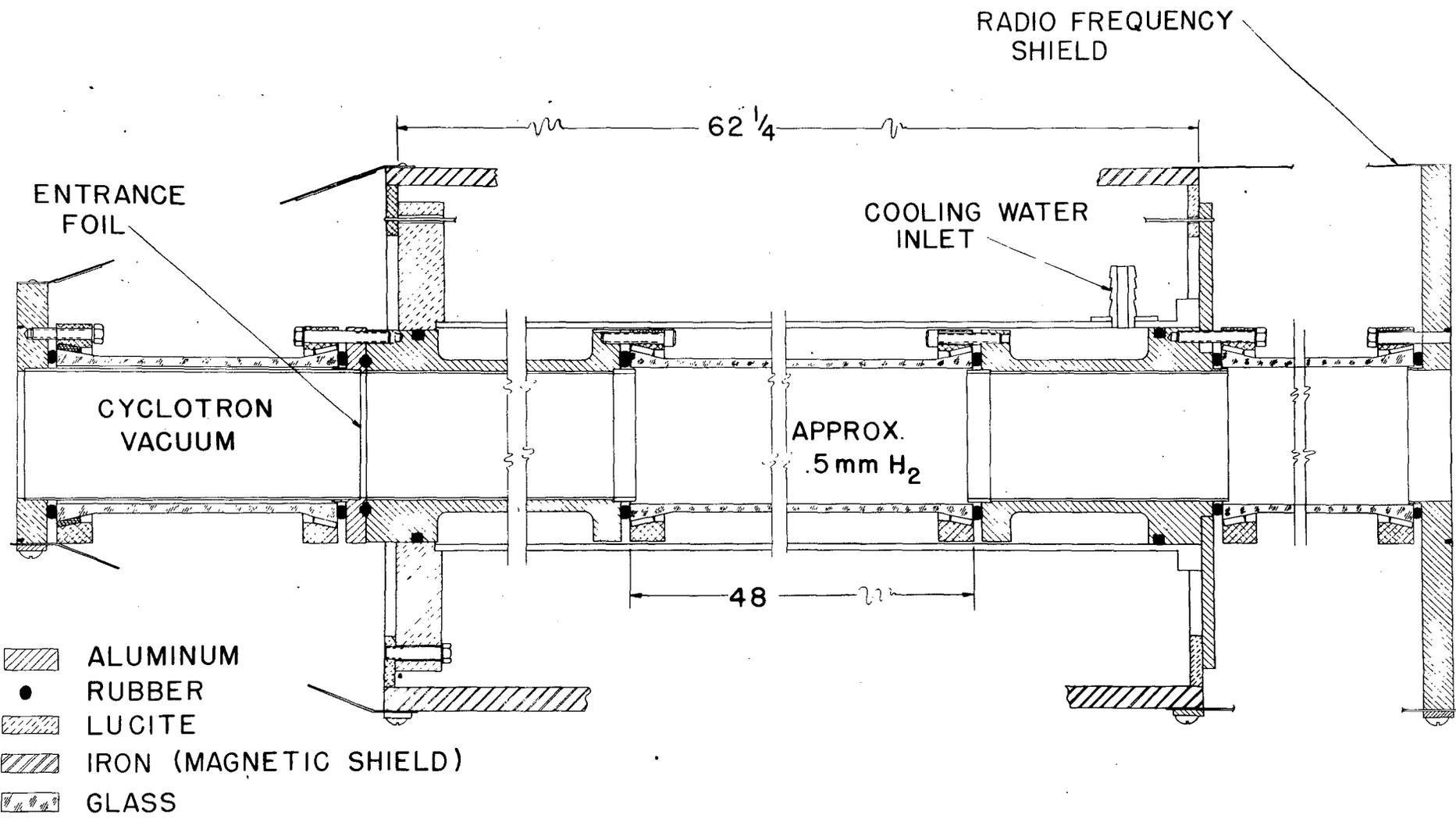
FIG. 2 CROSS SECTION OF MAGNETIC ARC LENS.
