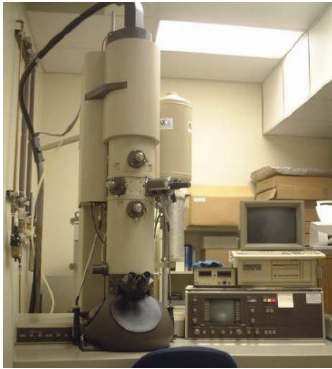
Fig. 2.9 FEI/Philips CM-20 conventional TEM.
