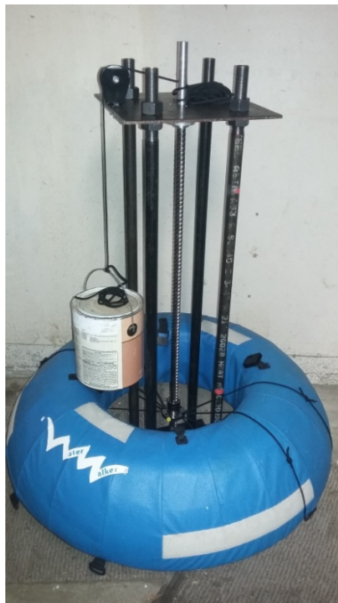
Figure 9. Physical prototype with paint can acting as a weight to be lifted.
