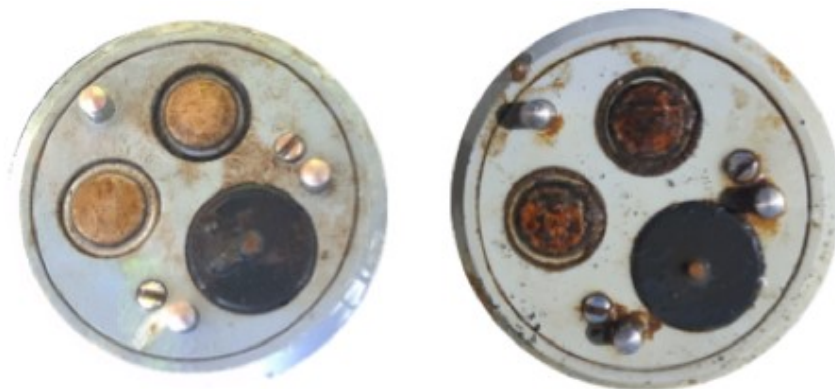
Figure 2.5: Pictures of different fouling conditions of the probe installed in low range application. a) One month of fouling in the first month since installation. b) One month of fouling after three months from installation.
