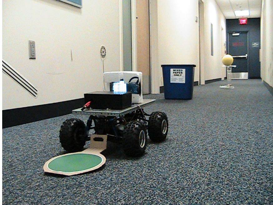
Figure 6.1: “Le Carl” Android based robot, which was constructed from the chassis of an R/C car. The task of the robot was to navigate to a visually salient target (bright yellow foam ball) while avoiding an obstacle (blue recycle bin) along the way. The robot’s position throughout the task was monitored by an overhead camera that tracked the position of the green marker.
