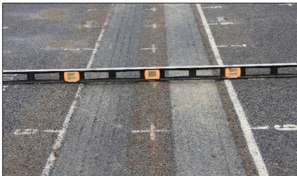
Figure 5.40: 701HC: View of rut at Station 8.
