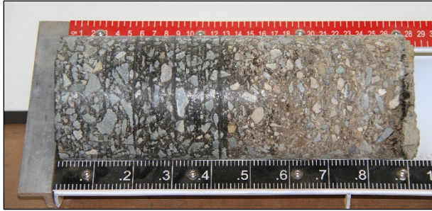
Figure 5.63: 700HB: Core taken in wheelpath.
