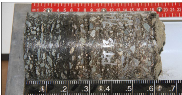
Figure 5.21: 704HB: Core taken in wheelpath.
