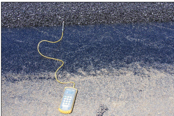
Figure 3.13: Temperature measurement with thermocouple.
