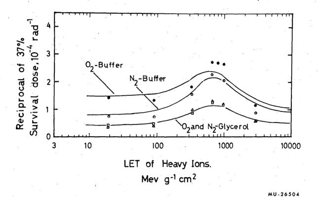
Fig. 7. Theoretical curves calculated by track-segment method.
