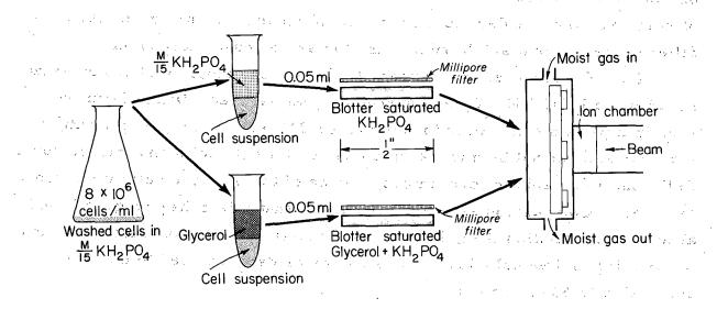
Fig. 1. Schematic diagram illustrating procedure used to control atmosphere and solution to which yeast were exposed during irradiation with heavy ions.
