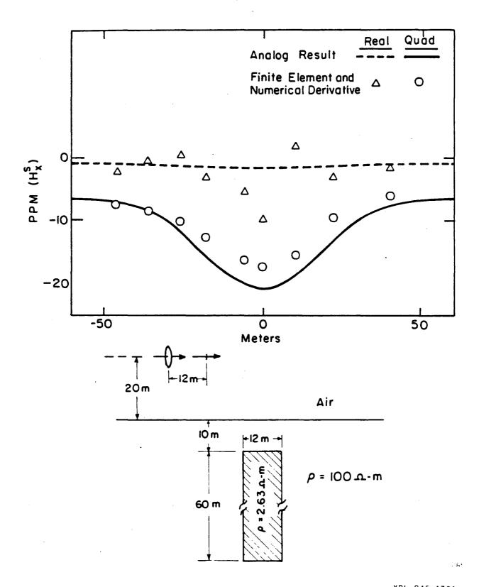
Figure 3. Numerical model result with the use of numerical derivative.
