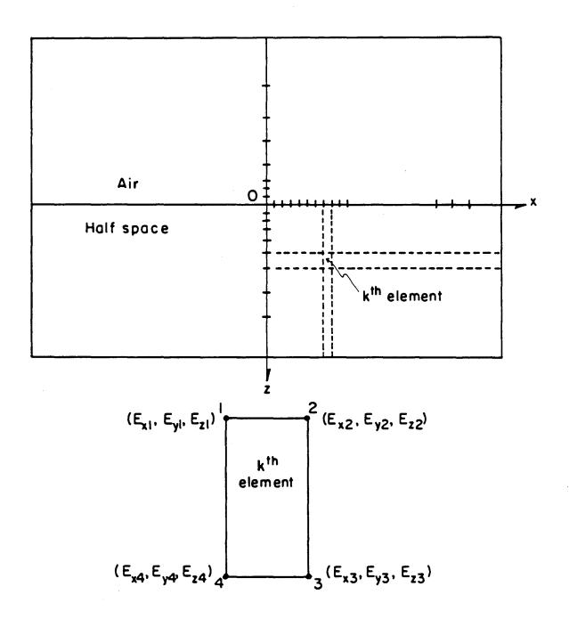
Figure 2. A finite element grid and notations used for the description of a rectangle.
