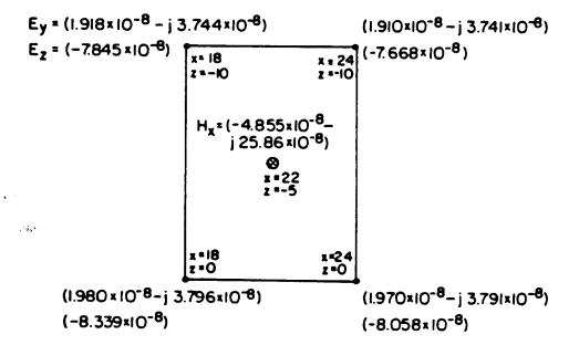
Notice that  $H_x$  is analytically obtained and displayed at the center of the rectangle. With the assumption that the electric field would behave linearly within the rectangle, one can numerically compute the secondary magnetic field  $H_x$  as
