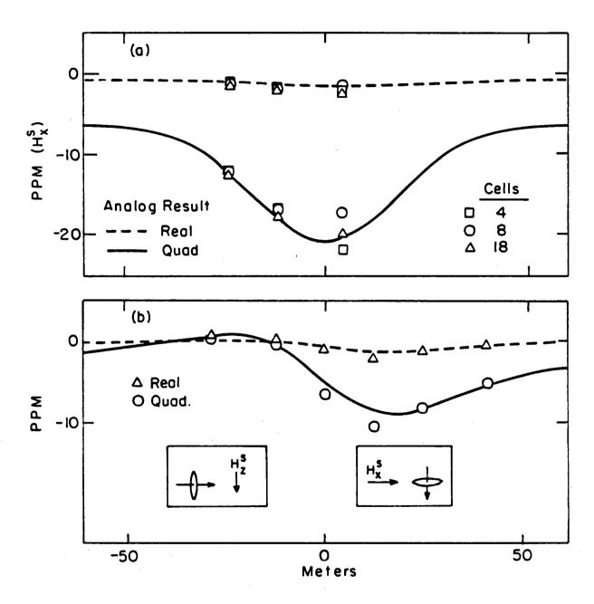
Figure 4.a Convergence test of the numerical solution.
