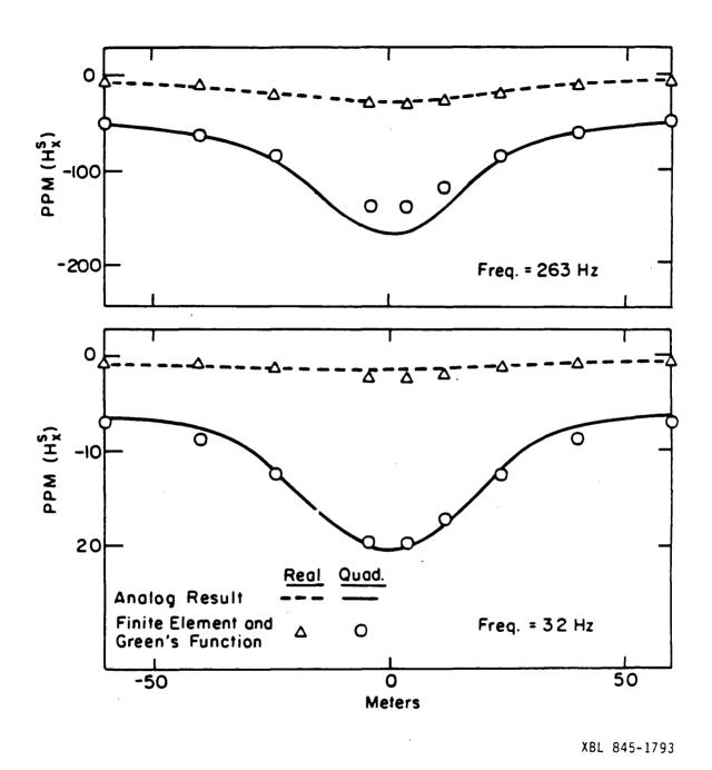
Figure 5. Comparison between analog result and numerical result with the use of Green's function.
