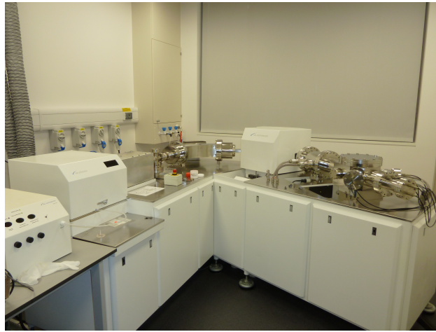
Figure 2.3: Multi-Collector Inductively Coupled Plasma Mass Spectrometer(MC-ICP-MS) is used to determine Tham Mai cave speleothems U - Th ages
