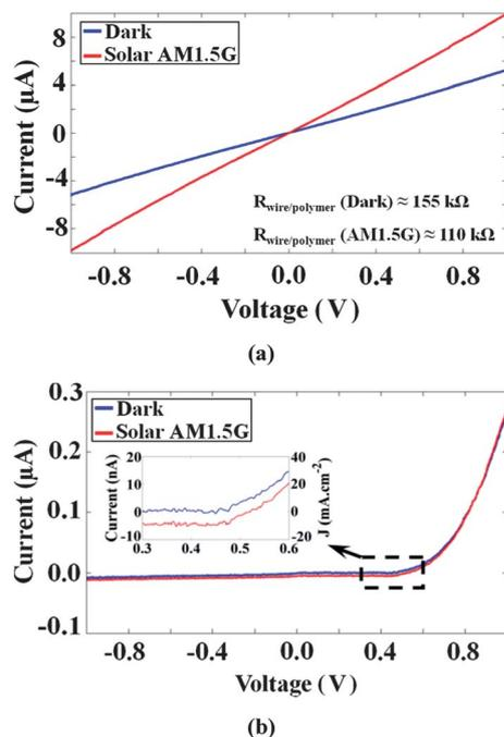
**Fig. 4** Measured  $I$ - $V$  data for a  $100 \mu\text{m}$  long CH<sub>3</sub>-terminated (a) p-type and (b) n-type Si microwire with a diameter  $\approx 1.5 \mu\text{m}$  aligned at the PEDOT:PSS:Nafion/glass border, in dark and under solar AM 1.5G illumination. As expected, ohmic behavior was observed at the p-Si microwire/polymer contact. A strong rectifying behavior was observed at the CH<sub>3</sub>-terminated n-Si microwire/polymer junction.
