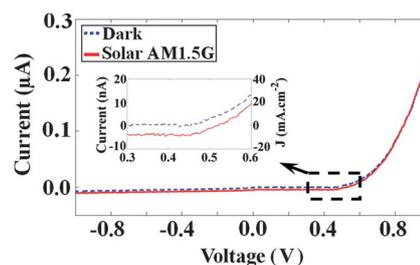
**Fig. 5** Measured  $I$ - $V$  response for a complete photoelectrosynthetic water splitting cell with  $\sim 100 \mu\text{m}$  long CH<sub>3</sub>-terminated p-Si and n-Si microwires with diameters of  $\sim 1.5 \mu\text{m}$ . The electrical character of the cell is dominated by the rectifying behavior at the CH<sub>3</sub>-terminated n-type microwire/polymer junction.
