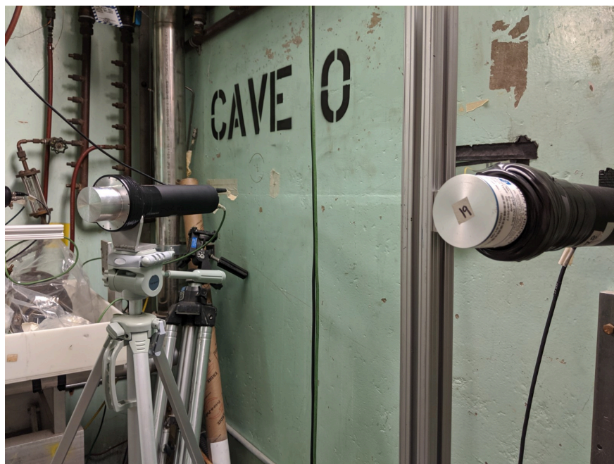
Figure 3.13: Photo of the EJ-309 neutron scintillation detectors used in the time-of-flight experiment. Pictured here are the detectors positioned at 0^{\circ} and 18.2^{\circ} .
