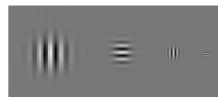
Figure 3: A Gabor function is constructed by multiplying a Gaussian function by sinusoidal function [Daugman, 1985]. We used five scales with eight orientations.
