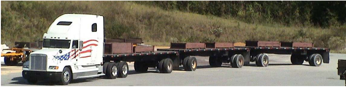
Figure 4.8: Triple trailer truck used to apply trafficking.
