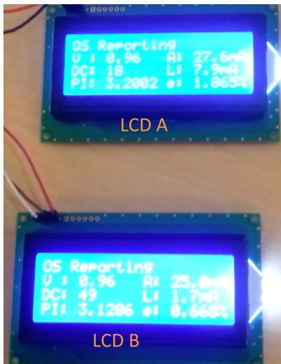
Fig. 13. A snapshot of the demo results after heating up Instance A (reported by LCD A). If the system is “designed for worst case”, it has to margin for scenario of Instance A and set DC = 18 . While our system shows its capability of reducing the margin and run at DC = 49 , as the scenario of Instance B.
