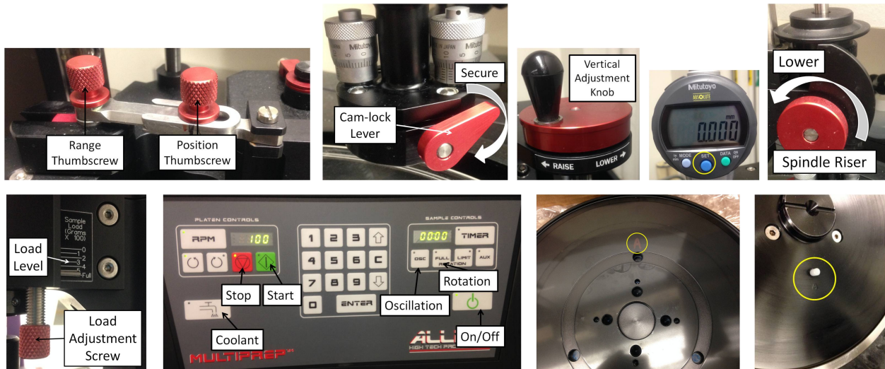
Figure A.3: Details of the lapping machine.
