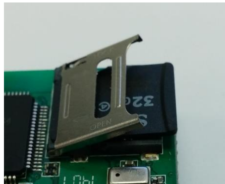
Figure 19: SD Card and Connector Implemented on Embedded System Node
