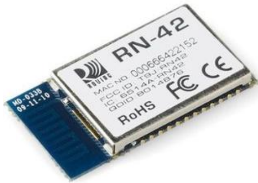
Figure 18: Roving Networks RN-42 Bluetooth Chip and Schematic [14]
