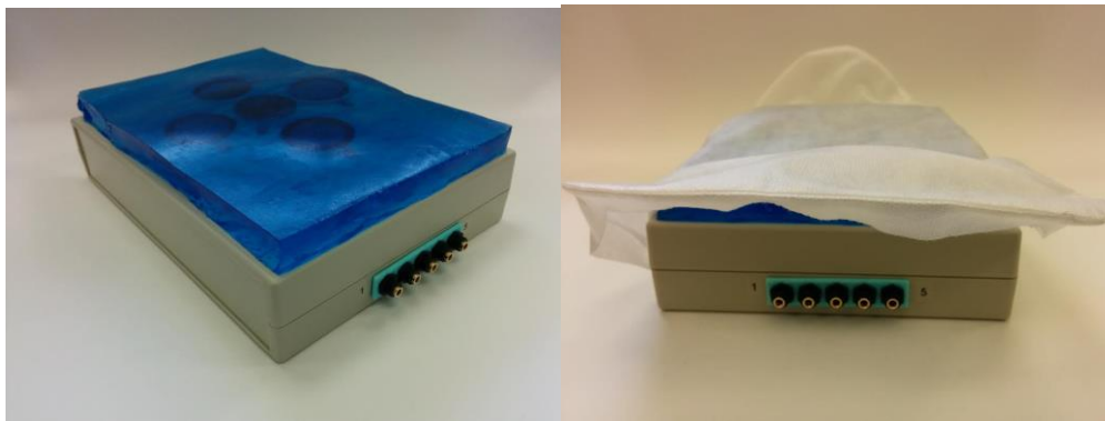
Figure 29: Acoustic Platform to Measure Data Safely From Infants
