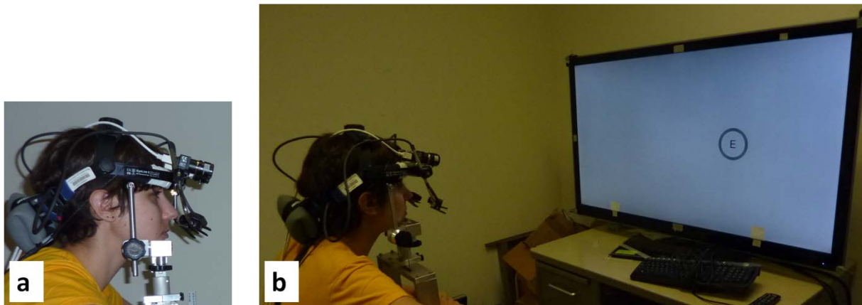
Figure 3-3. (a) Subject's head secured in chinrest during calibration. (b) Example of display setup during calibration. Subject is at 100 cm from display.
