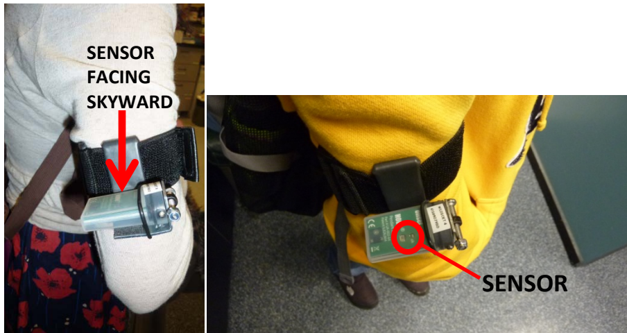
Figure 2-1. Two subjects wearing the armband with light sensor attached to the custom pedestal.
