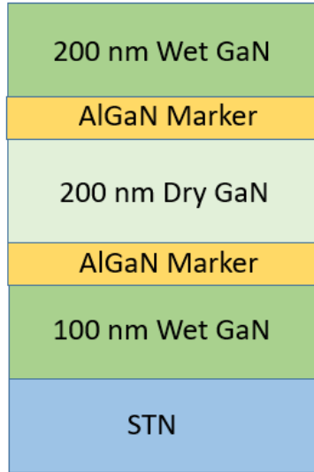
Figure 15. Epitaxial structure for Samples D and E. Sample D was grown at 720 °C, and Sample E was grown at 765 °C.
