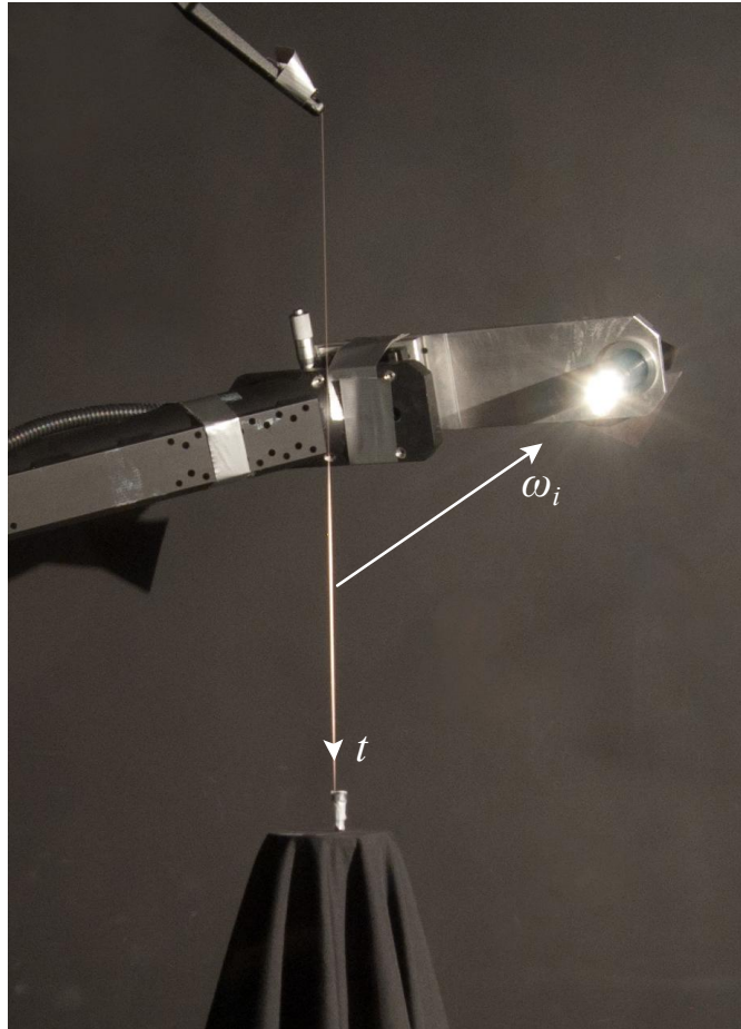
Figure 5.17: An illustration of the acquisition setup for measuring the BRDF of threads.
