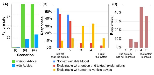
Figure 6.7: (A) We report the failure rate with and without advice inputs in the following three scenarios on a Carla simulator. (B-C) We also report the responses from our human study for the questions: (B) "How much do you trust this system?", and (C) "To what level has the system improved with the human-to-vehicle advice?". Answers were measured on a 1-5 Likert scale.
