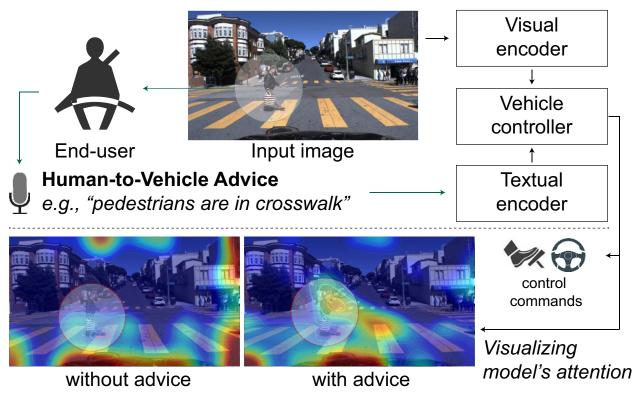
Figure 5.1: Our model takes human-to-vehicle advice as an input, *i.e.* "pedestrians are in crosswalk", and grounds it into the vehicle controller, which then predicts a sequence of control commands, *i.e.* a steering wheel angle and a vehicle's speed. Our driving model also provides a visual explanation in the form of attention - highlighted regions have a direct influence on the function being estimated. Visualizing attention maps helps the end-users acknowledge the acceptance of their advice.
