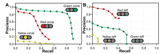
Figure 2.4: Performance evaluation of our coarse-grained detector in terms of two widelyused metrics: precision and recall. For red, green, and yellow circles, see A. For others, see B.
