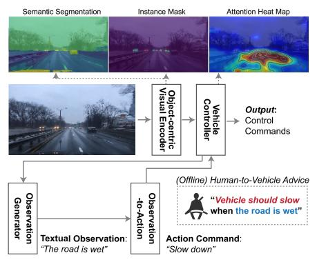
Figure 6.1: Our model consists of four main parts: (1) an object-centric visual encoder built upon a semantic segmentation model, (2) an observation generator, which generates textual observation about the scenes ("The road is wet"), (3) an observation-to-action module, which maps a visual scene description to a (high-level) action command ("Slow down"), and (4) a vehicle controller conditioned on the generated action command.
