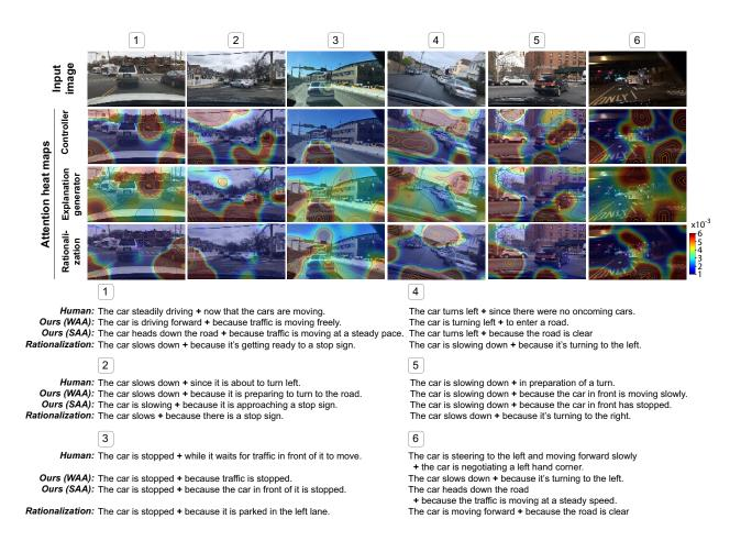
Figure 4.6: Example descriptions and explanations generated by our model compared to human annotations. We provide (top row) input raw images and attention maps by (from the 2nd row) vehicle controller, textual explanation generator, and rationalization model (Note:  $(\lambda_c, \lambda_a) = (100, 10)$  and the synthetic separator token is replaced by '+').
