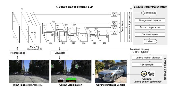
Figure 2.2: An overview of our proposed model. It can be understood in three parts: (i) a coarse-grained detector that utilizes the deep neural perception network architecture called SSD (Single-Shot multi-box Detector [50]), (ii) a spatiotemporal filtering, and (iii) a vehicle controller. To demonstrate the feasibility of applying our model to self-driving cars, we use an instrumented autonomous vehicle which uses the output of our model as an input to control its dynamics.
