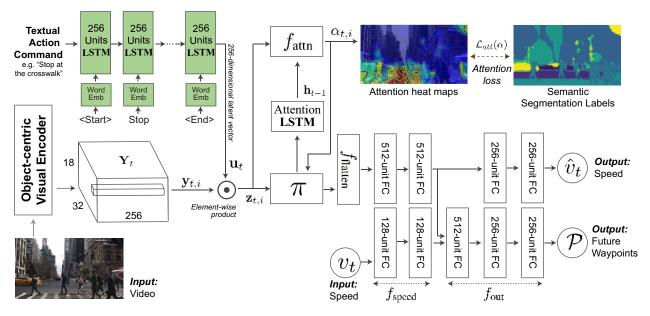
Figure 6.4: The detailed overview of our goal-conditioned Vehicle Controller. We take an action command in natural language as an input and ground it into the controller. Our model adopts spatial attention mechanism  $\pi$ , which guides where the controller looks. Conditioned on the attended feature and the current speed  $v_t$ , our model outputs future trajectory  $\mathcal{P}$  and speed  $\hat{v}_t$ . For details, see Section 6.2.2.
