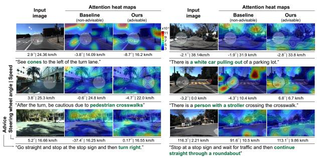
Figure 5.4: Attention heat maps comparison. We provide input raw images and attention heat maps generated by the existing attention-based driving model [37] (Baseline column), and our model trained with all types of advice together (Ours column). We highlight key object-centric words (as appropriate row 1 & 2), *e.g.* cones and a white car pulling out, in green as well as corresponding salient objects in a green circle overlaid on images.
