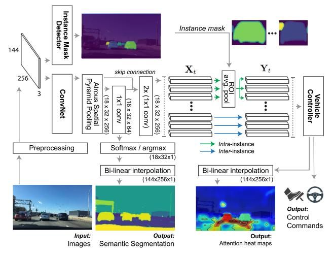
Figure 6.3: The detailed overview of our *Object-centric Visual Encoder* that is built upon an instance mask detector and a semantic segmentation model, both of which provide pixel-wise category predictions from images along with delineating the boundaries of object.
