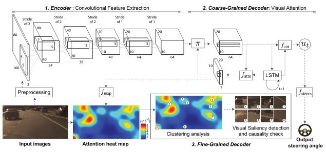
Figure 3.1: Our model predicts steering angle commands from an input raw image stream in an end-to-end manner. In addition, our model generates a heat map of attention, which can visualize where and what the model sees. To this end, we first encode images with a CNN and decode this feature into a heat map of attention, which is also used to control a vehicle. We test its causality by scrutinizing each cluster of attention blobs and produce a refined attention heat map of causal visual saliency.
