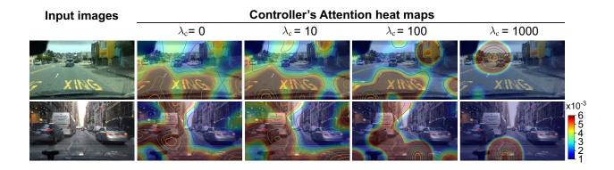
Figure 4.5: Vehicle controller's attention maps in terms of four different entropy regularization coefficient  $\lambda_c = \{0, 10, 100, 1000\}$ . Red parts indicate where the model pays more attention. Higher value of  $\lambda_c$  makes the attention maps sparser. We observe that sparser attention maps improves the performance of generating textual explanations, while control performance is slightly degraded.
