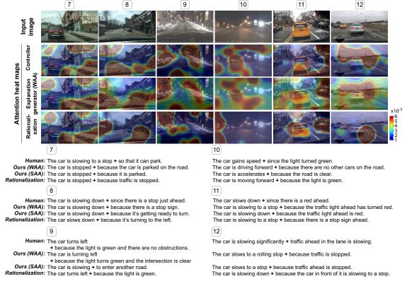
Figure 4.7: Examples of descriptions and explanations. In this experiment, we use  $(\lambda_c, \lambda_a)$ as (100,10). A synthetic separator token is replaced by '+'.
