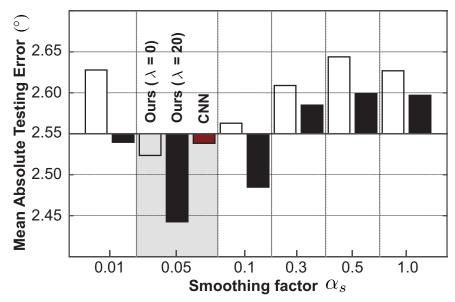
Figure 3.4: Effect of applying a single exponential smoothing method over various smoothing factors from 0.1 to 1.0. We use two different penalty coefficients  $\lambda \in \{0, 20\}$ . With setting  $\alpha_s = 0.05$ , our model performs the best. *Data*: Comma.ai [19]
