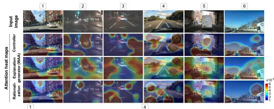
Human: The car isn't moving + because the light hasn't turned green yet. Ours (WAA): The car is stopped + because the light is red. Ours (SAA): The car is stopped + because the light is red.
