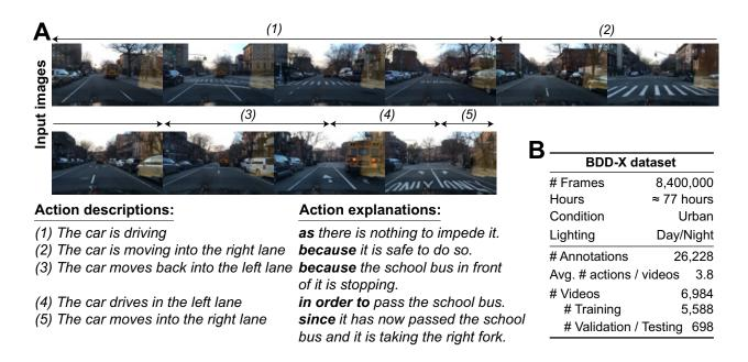
Figure 4.3: (A) Examples of input frames and corresponding human-annotated action description and justification of how a driving decision was made. For visualization, we sample frames at every two seconds. (B) BDD-X dataset details. Over 77 hours of driving with time-stamped human annotations for action descriptions and justifications.
