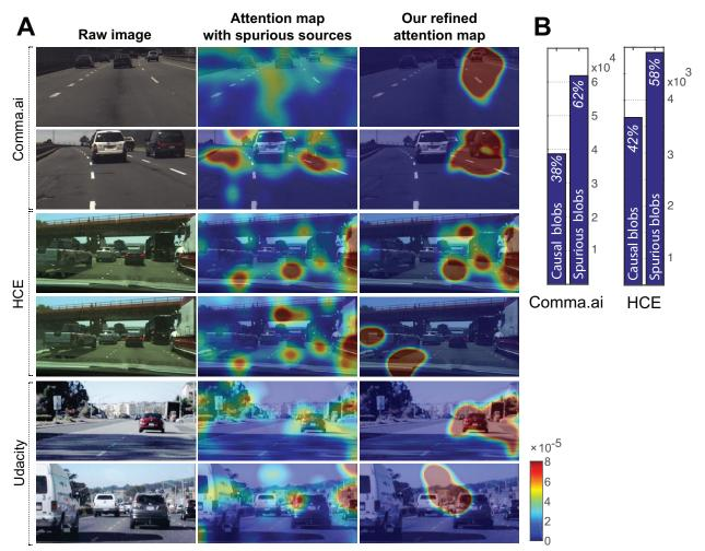
Figure 3.5: (A) We illustrate examples of (left) raw input images, their (middle) visual attention heat maps with spurious attention sources, and (right) our attention heat maps by filtering out spurious blobs to produce simpler and more accurate attention maps. (B) To measure how much the causal filtering is simplifying attention clusters, we quantify the number of attention blobs before and after causal filtering.
