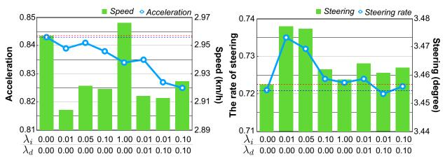
Figure 5.6: Control performance comparison with different sets of hyperparameters  $(\lambda_d, \lambda_i)$  (see Equation 5.2). Along with proportional prediction errors (green bar), we also visualize derivative errors (blue line). We report the median value of absolute error.
