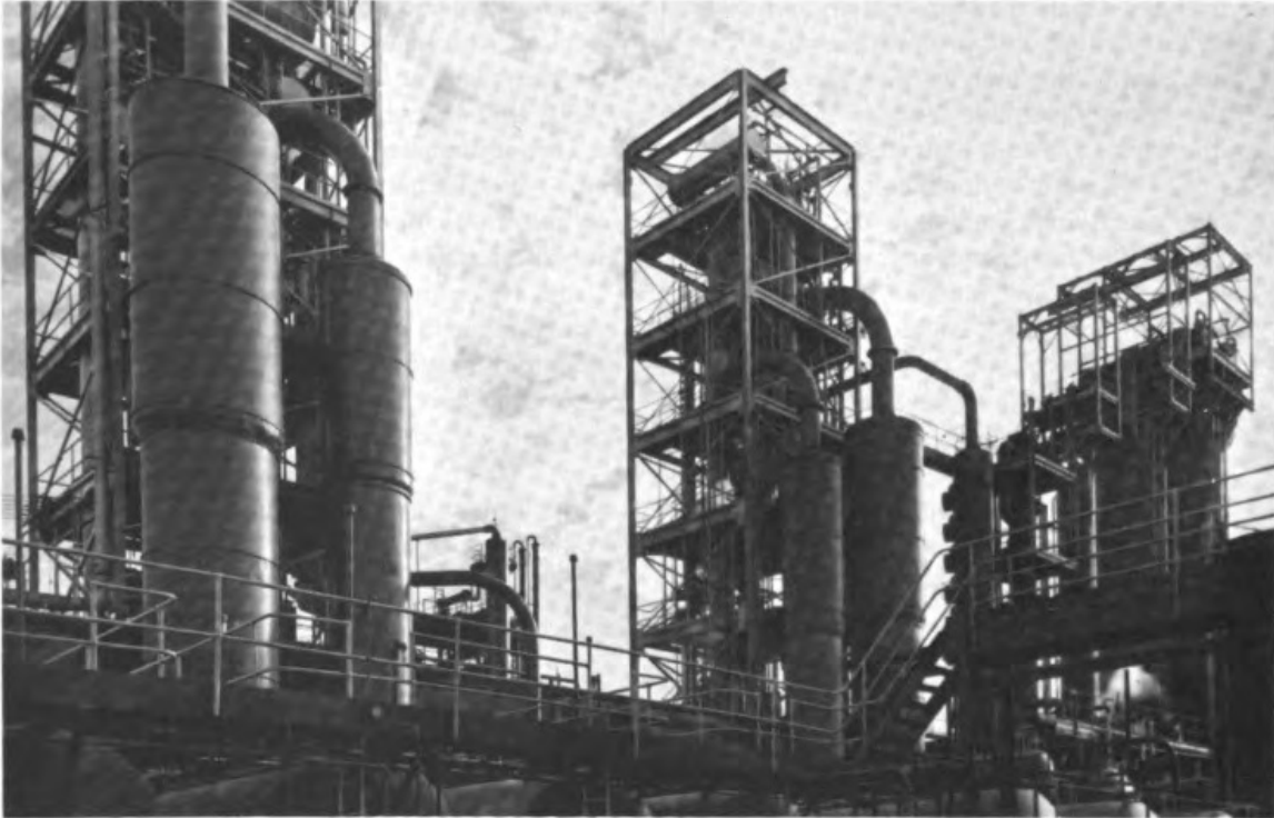
Figure 12-31 Three sets of primary-secondary column distillation units for styrene at the Dow Midland Plant. ( Dow Chemical USA, Midland, Michigan. )
