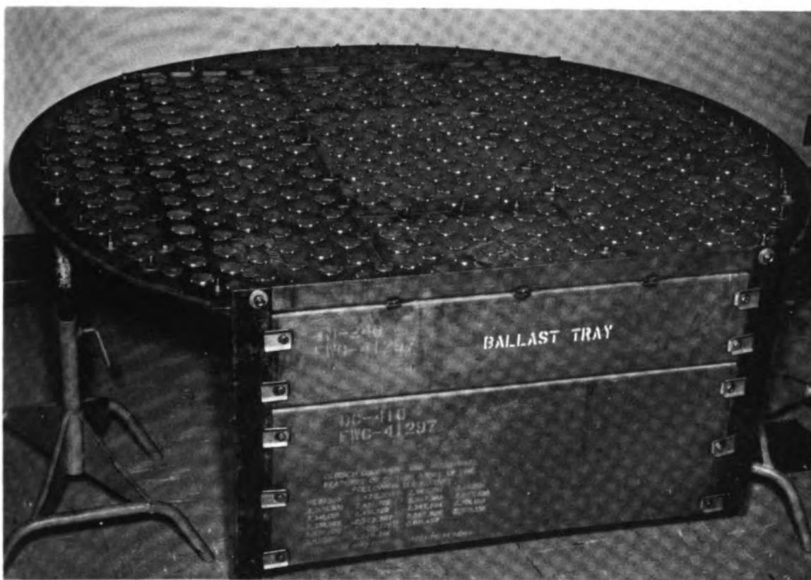
Figure 4-12 A 1.8-m-diameter valve-cap tray. (Fritz W. Glitsch & Sons, Inc., Dallas, Texas)
