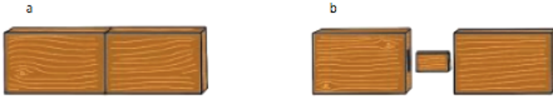
Figure 31: a) Edge joint. b) Edge joint connected with loose tong and dowels. Image by author.
