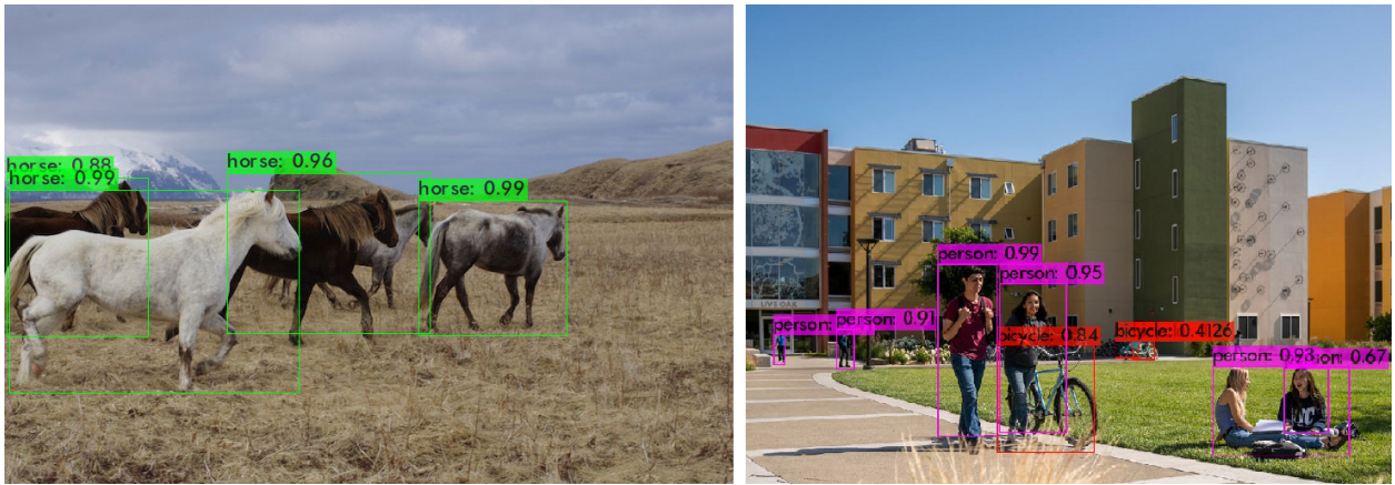
Figure 1.1: Example outputs of the YOLOv3 Object Detection System, the predicted category is accompanied with a confidence score. The maximum possible score is 1.00.
