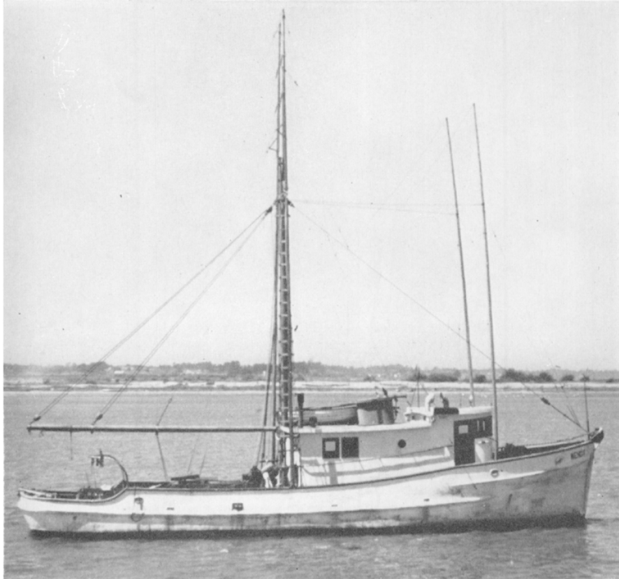
FIGURE 8. Salmon trolling boat at Eureka. Outrigger poles made fast at the mast. Bow poles forward of the house. Photograph by D. H. Fry, Jr., July, 1948.
