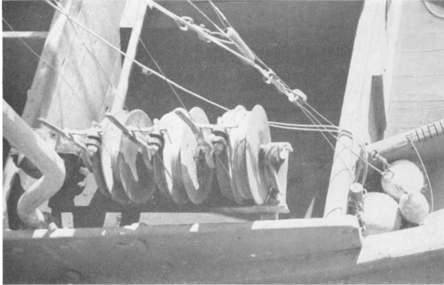
FIGURE 10. The three portside spools of the gurdy in the stern of a salmon trolling boat. Cannon ball sinkers at the extreme right. Photograph by D. H. Fry, Jr., 1949.
