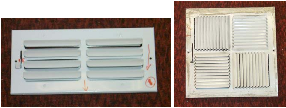
Figure 3. Examples of registers used in flow hood test apparatus
