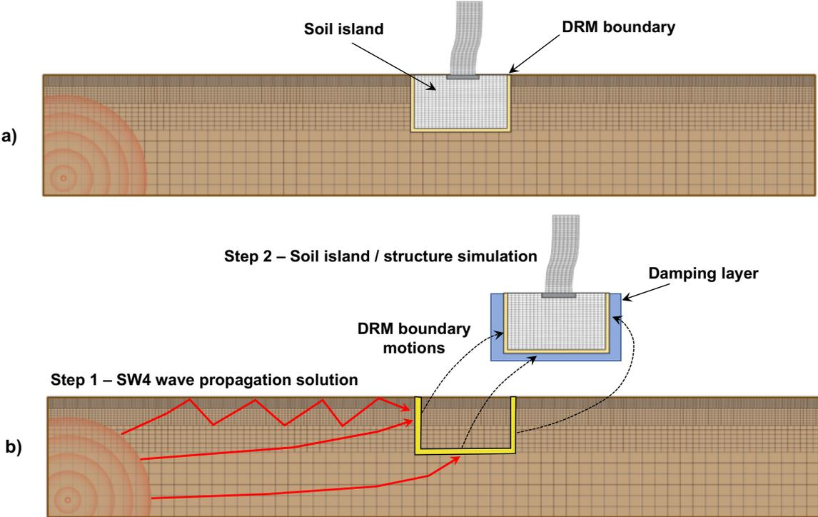
**Figure 5. Global-local model coupling through the Domain Reduction Method. a) Conceptual embedding of soil-structure domain within the global geophysics grid; b) practical implementation as a two-step solution where DRM boundary motions are applied to the DRM boundary of the soil-structure domain model.**
