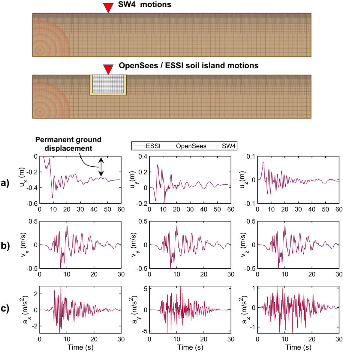
**Figure 14. Comparison of simulated earthquake motions at the surface of the ground for a near-fault site (subdomain 53 in Figure 11). a) Ground displacement time histories; b) ground velocity time histories; c) ground acceleration time histories.**
