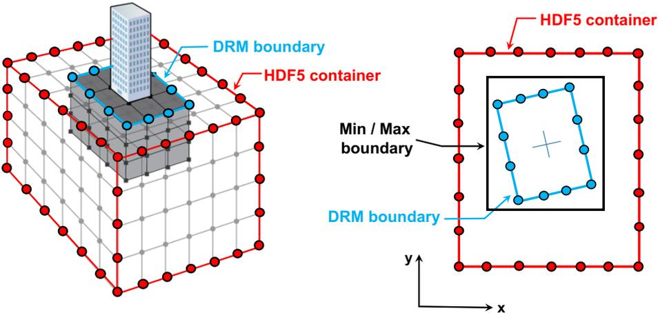
**Figure 10. Ground displacement and acceleration fields interpolated to the DRM boundary via spline function generated continuous acceleration and displacement fields.**
