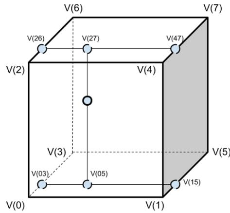
**Figure 9. Spline function representation of continuous field variables based on discrete grid point values.**
