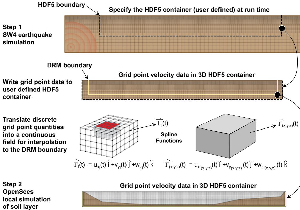
**Figure 7. Computational workflow for DRM-based coupling between regional geophysics and local engineering simulation codes.**
