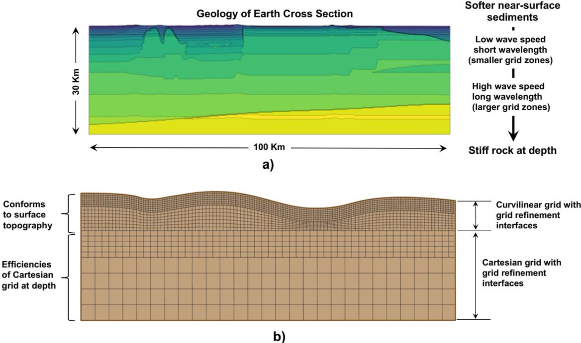
**Figure 3. Mesh refinement to represent the depth-dependent properties of the earth. a) Variation of geologic properties in a cross-section of the SFBA model of Figure 2; b) schematic of SW4 curvilinear and Cartesian grids with mesh refinement boundaries.**
