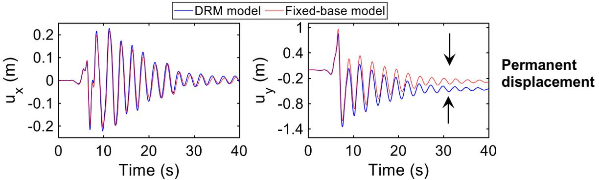
**Figure 16. Roof displacement time history of the twenty-story building in fault-parallel ( $U_x$ ) and fault-normal ( $U_y$ ) directions. Large fault-normal ground pulse results in significant inelastic deformation of the building.**
