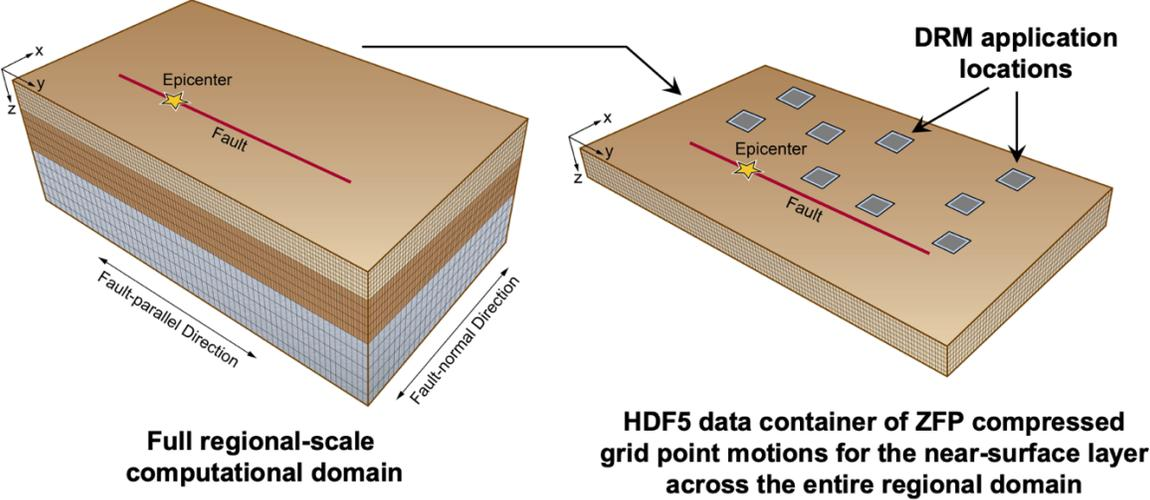
**Figure 8. Compression and storage of ground motion data from a near-surface volume of a regional scale geophysics model allows DRM coupling at any selected site.**
