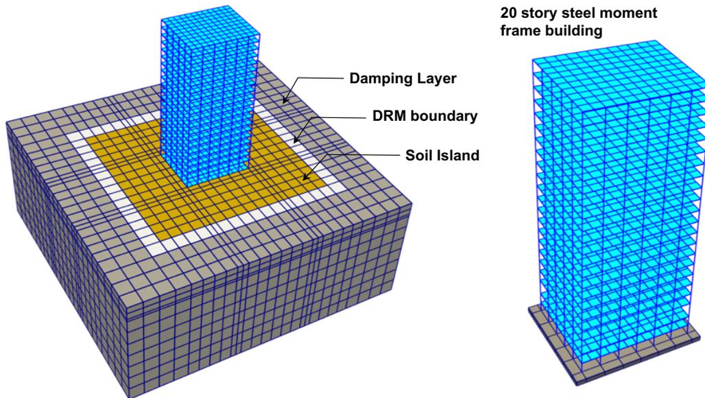
**Figure 12. Local engineering system model of soil island and twenty story steel moment frame building in the OpenSees program.**
