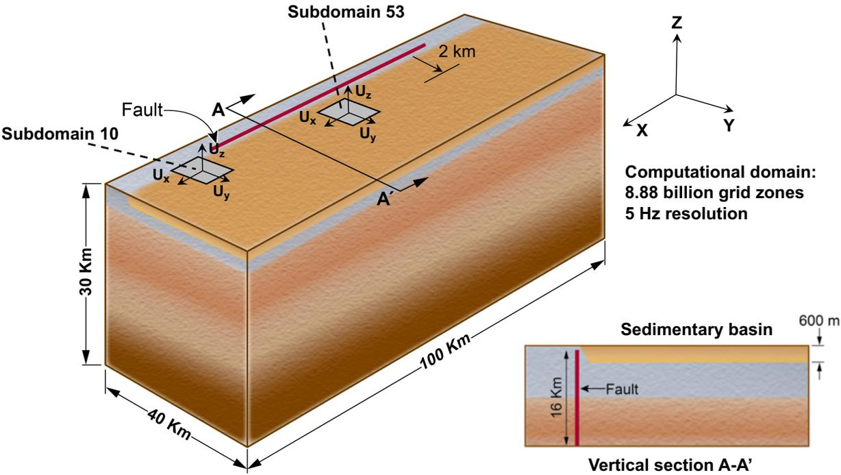
**Figure 11. A representative regional domain with a strike slip earthquake fault, subdomains for HDF5 data containers indicated by grey boxes.**
