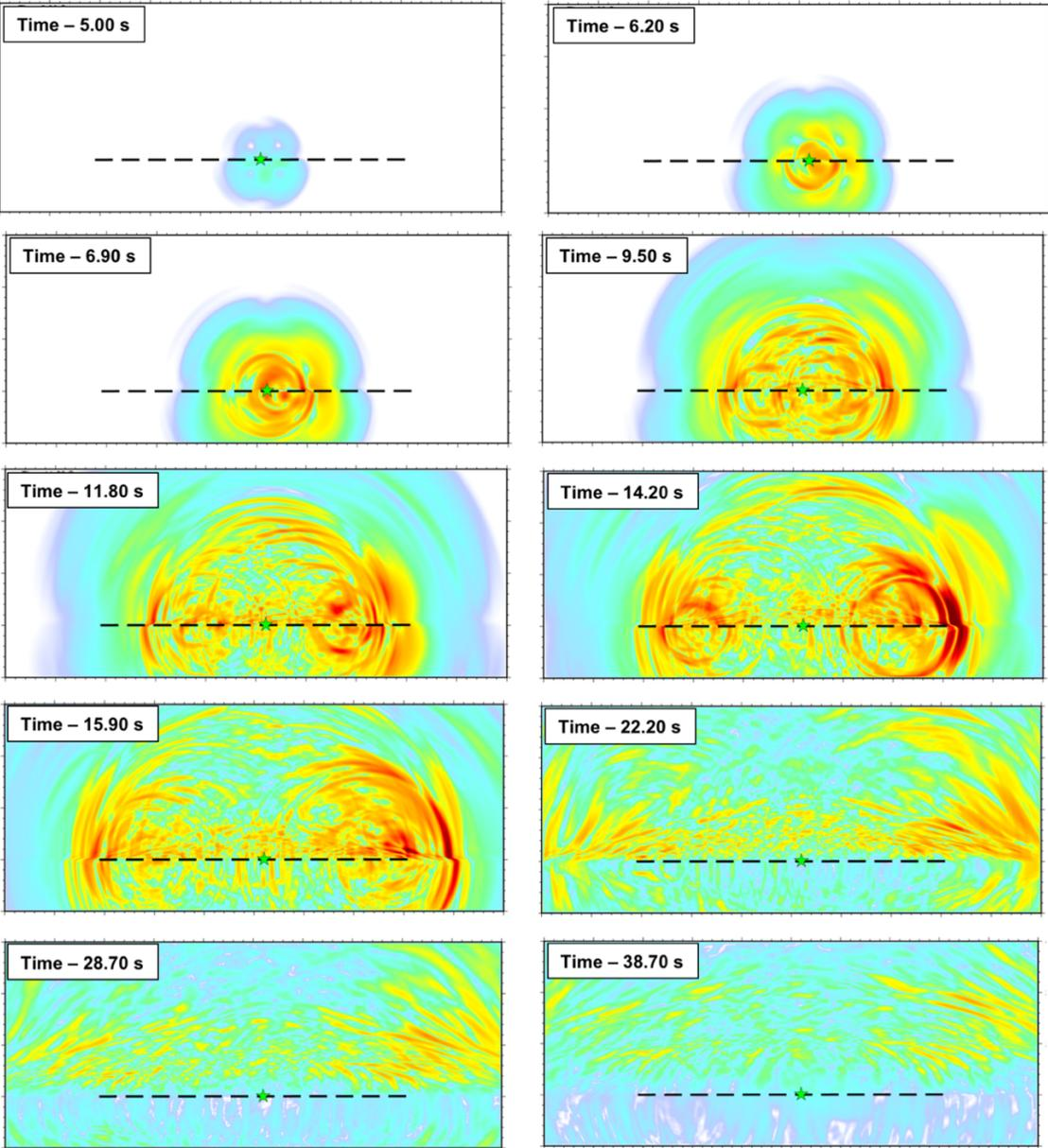
**Figure 13. Simulation of a M7 earthquake rupture with SW4 in plan view, snapshots of seismic wave propagation at selected instants in time.**
