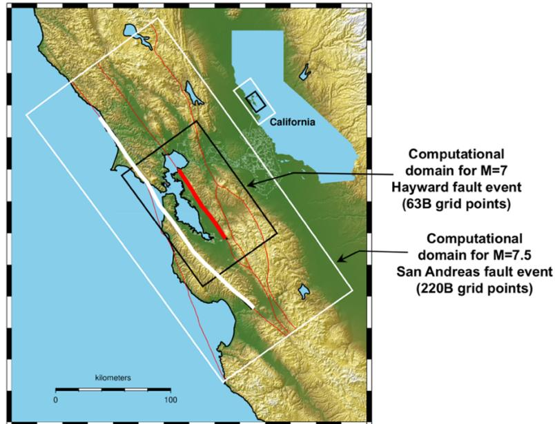
**Figure 2. Regional simulation domains for a M7 Hayward fault earthquake where the thick red line shows fault rupture length, and a M7.5 San Andreas fault earthquake where the thick white line shows fault rupture length.**
