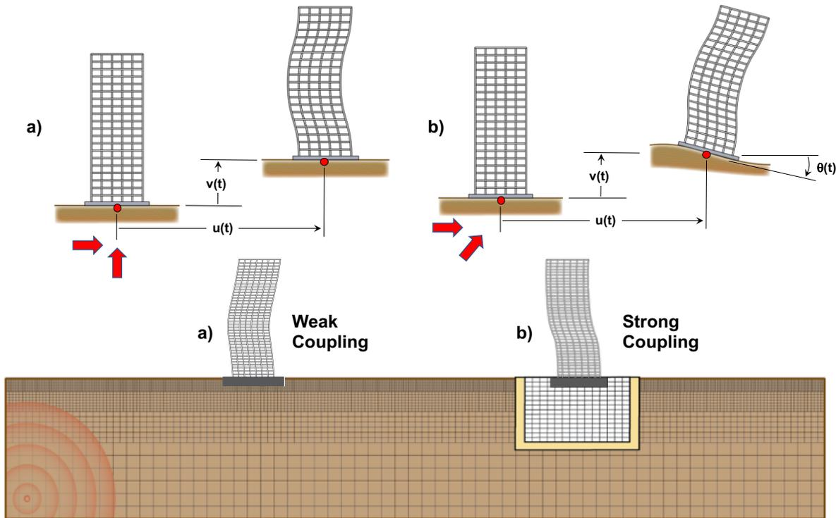
**Figure 4. Options for coupling regional geophysics and local engineering system models in EQSIM. a) Weak coupling where ground motions from a point on the ground surface are applied directly to building model resulting in horizontal and vertical translations of building; b) strong coupling where soil-structure-interaction and complex incident seismic waveforms are fully represented and building translates and rocks/rotates.**
