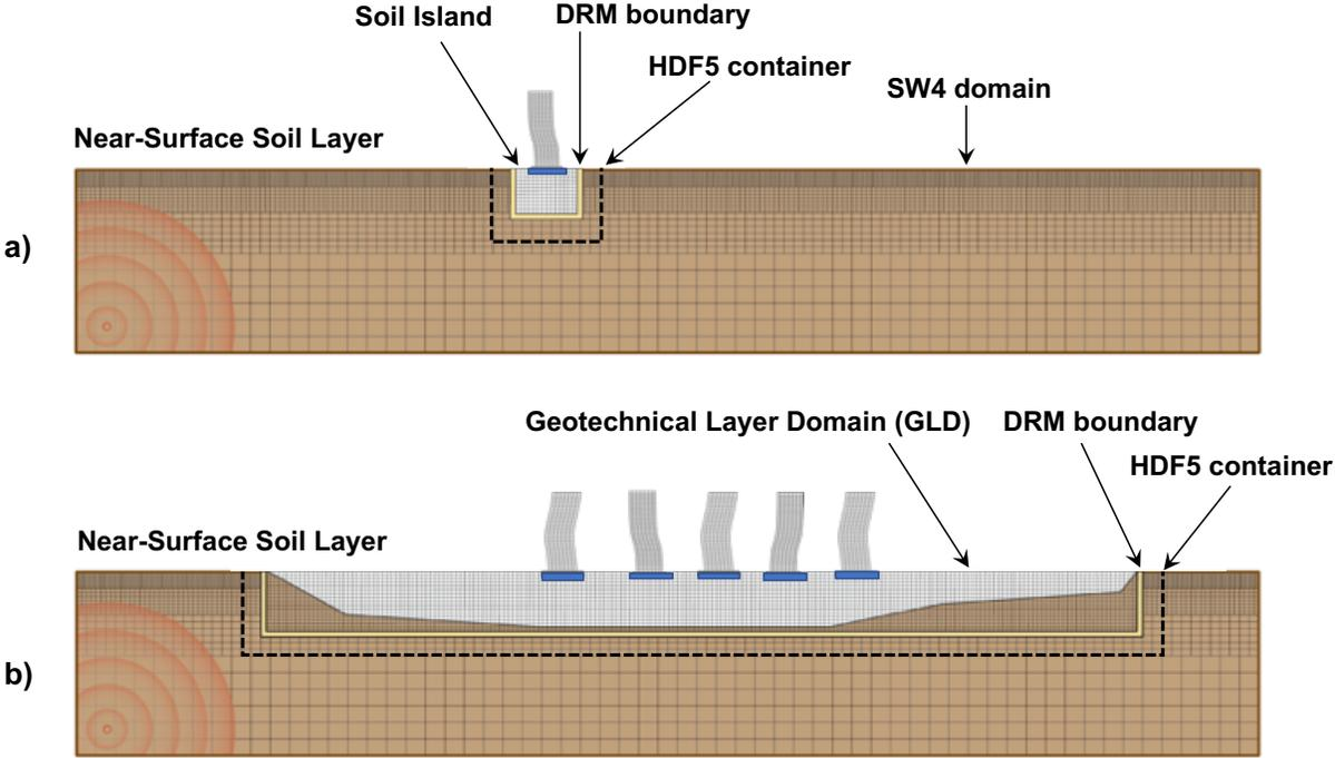
**Figure 6. Applications of the DRM-based code coupling. a) Representation of soil island - building system; b) representation of an extended geotechnical soil layer.**
