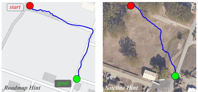
Fig. 9: ViKiNG can use geographic hints in the form of a schematic roadmap or a satellite image. Providing roadmap hints encourages ViKiNG to follow marked roads (left); with satellite images, it is able to find a more direct path by cutting across a meadow (right).
