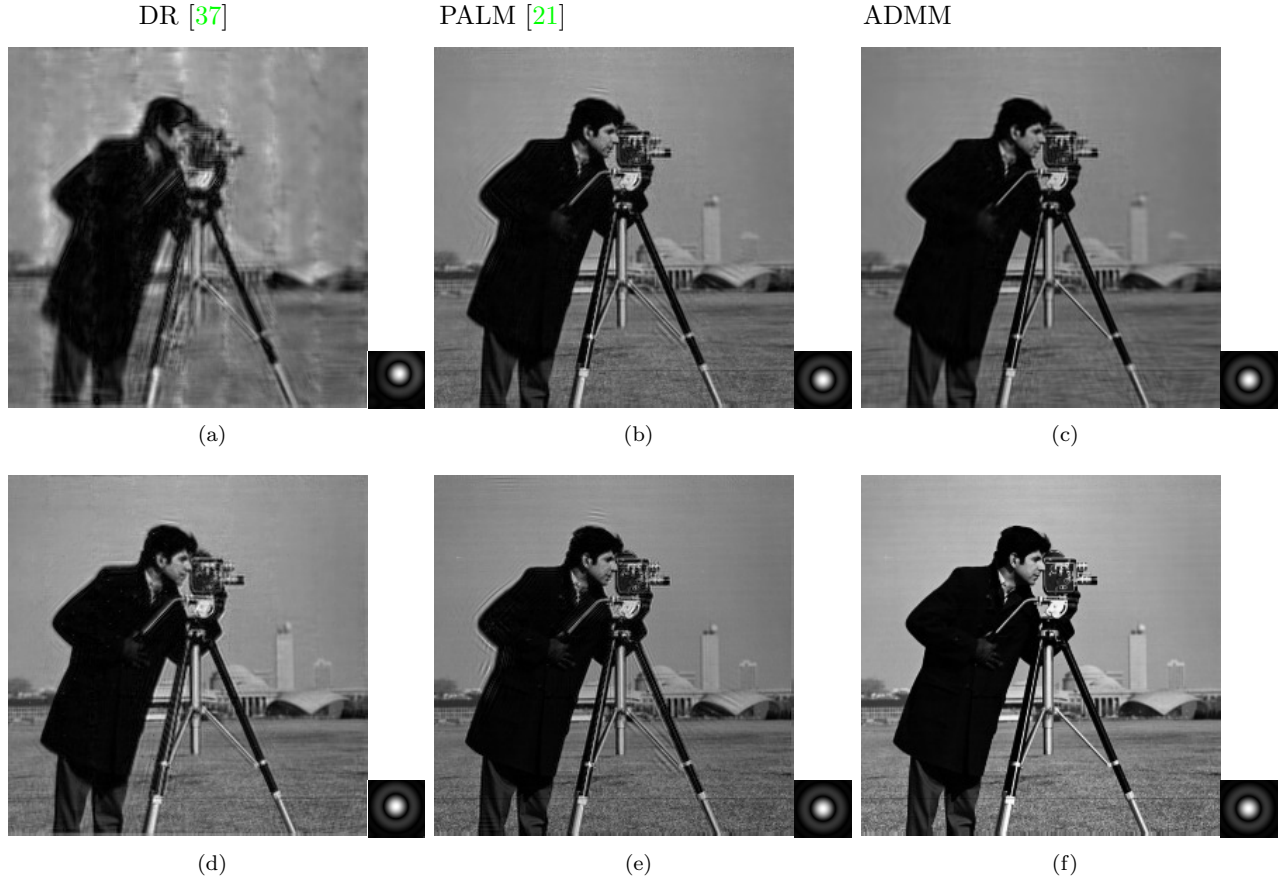
FIG. 7. Results of DR [37], PALM [21] and ADMM (Algorithm 1) with random-lattice scanning for Poisson noisy data. Peak level \eta = 0.1 (top), \eta = 1 (bottom). \beta = 0.5, 0.2 for Algorithm 1 with \eta = 0.1, 1 , respectively. All compared algorithms stop when the iteration number reaches Iter_{Max} = 300 .
