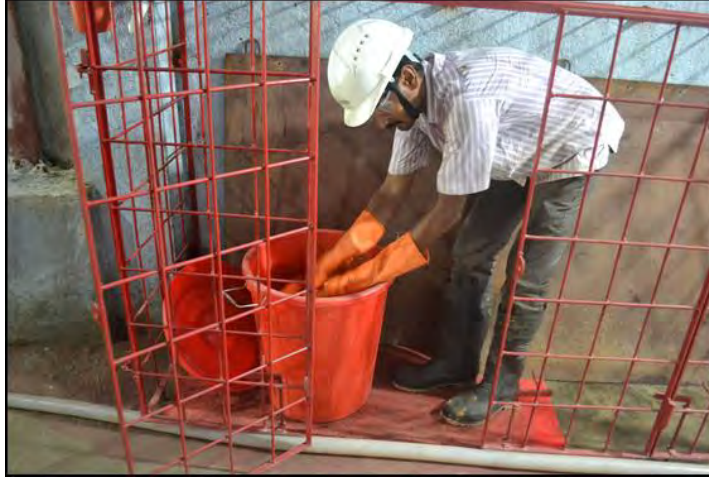
Fig. 14.12 Rathin, one of the locally trained plant operators, is safely storing sludge into the on-site cage, using proper personal protective equipment (PPE)
