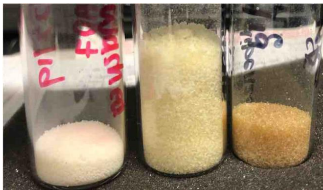
Figure 23: Pure XAD resin (left), XAD resin + nitrobenzene (middle), XAD resin + nitrobenzene + crown ether (right)
