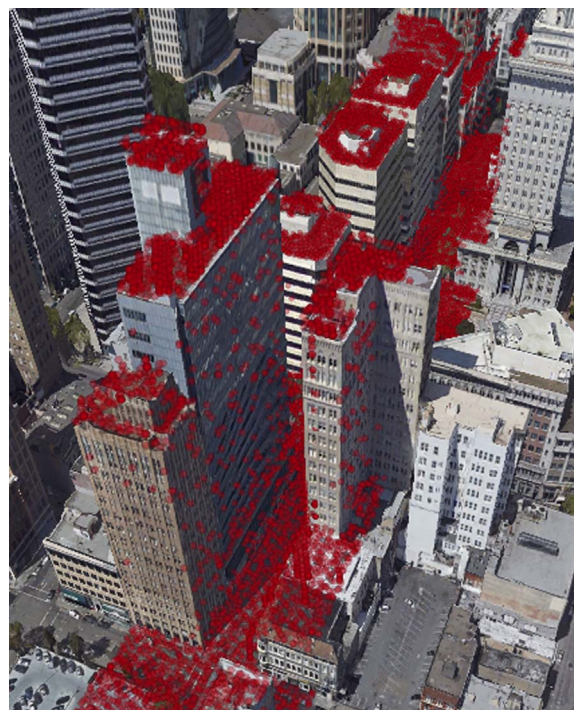
Fig. 11. Overlay of USGS lidar data on a portion of 14th Street in Oakland in Google Earth’s 3D structures view. Imagery © Google.
