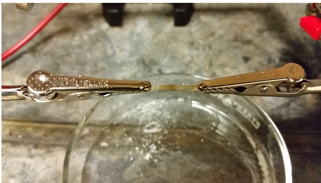
Figure D.3: To impregnate the salt or metal of interest, a filament is connected to a power supply via alligator clips, and salt deposited on the surface. A current of up to 20 A heats the filament to an orange-white color for 1 min, impregnated atoms. This procedure is performed inside a fume hood.
