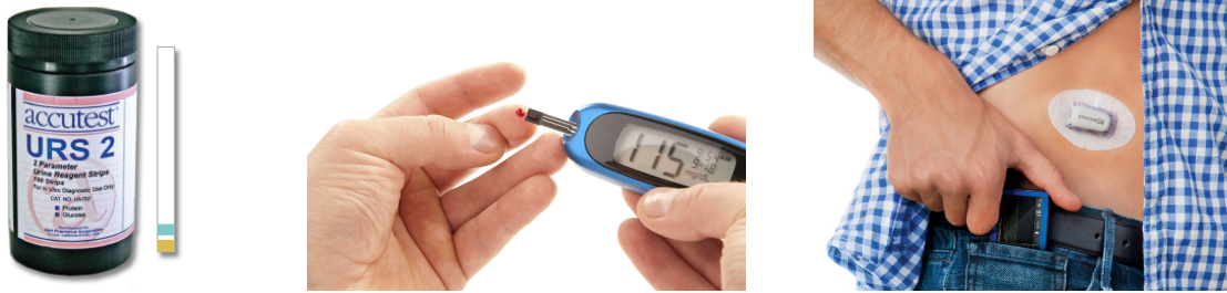
Figure 1.5: Examples of the tools for measuring BG. (left) Urine glucose test strips. (center) Finger-stick BG (FSBG) meter. (right) Continuous glucose monitor (CGM). The CGM consists of a sensor (white patch), a transmitter (round and grey), and a receiver (blue device placed in pocket). Urine test strips for BG measurement have been replaced by FSBG meters. FSBG meters may suffer a similar demise as CGMs become more comfortable, more accurate, and more affordable. Newer CGMs no longer require calibration with FSBG meters. Images from [18–20], used without permission.
