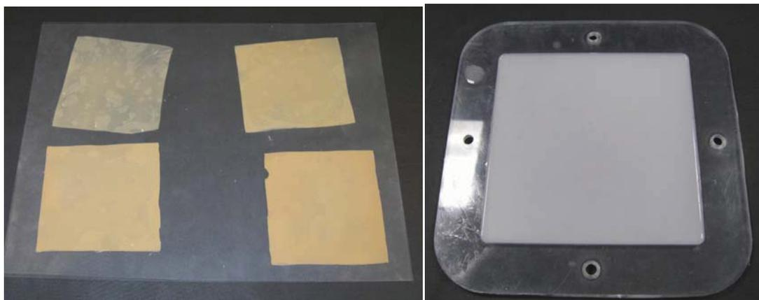
**Figure 4 Examples of Epidermal phantoms (left) and Dermal phantom (right) produced by this process. The epidermal phantoms, shown here, range from 90 to 500 micron. The dermal example is 1.93 mm thick.**
