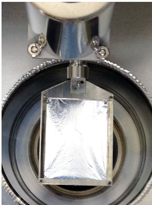
Fig. 9. The thin foil energy degrader used at the Michigan Ion Beam Laboratory for control of the implantation range of a light ion beam during multi-ion irradiation through foil rotation. The holder is shown with a 2.6 \mu\text{m} aluminum foil loaded and held taut by a crimp inside the holder frame.
