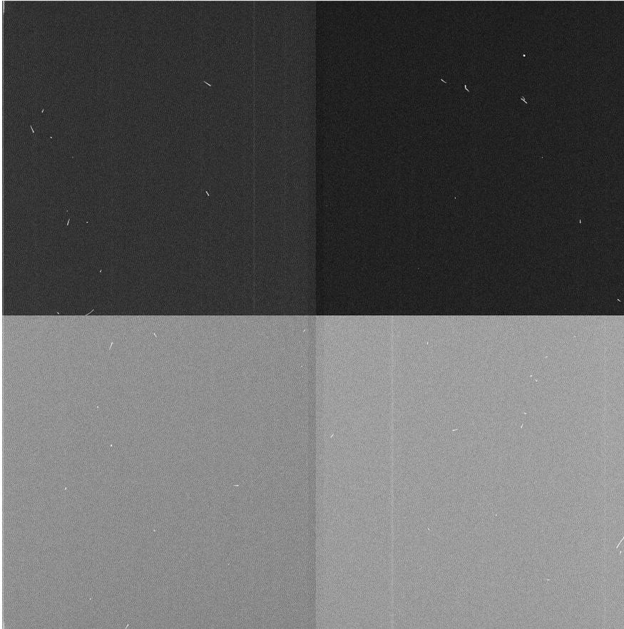
Figure 4.1: A bias frame taken with the LBNL  $4x \times 4k$  CCD. The image was read out using four amplifiers and hence, the four quadrants display different bias levels. Note the bright streaks in the image due to cosmic rays incident upon the CCD during the exposure.
