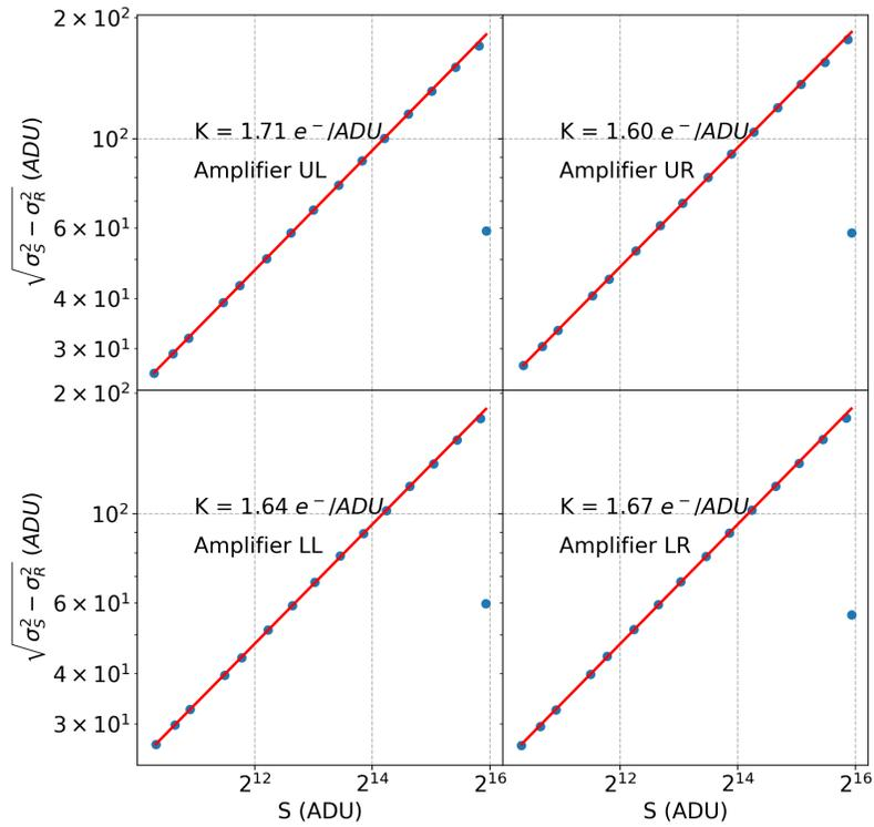
Figure 4.2: The photon-transfer curve for the LBNL 4k×4k CCD. The gain is estimated from the horizontal intercept of  $\log S$  vs  $\log(\sqrt{\sigma_S^2 - \sigma_R^2})$  line. The blue points represent the measurements, while the red curve is the line that best fits the data. The data point on the far right for every quadrant is at saturation and is not used in the fit.
