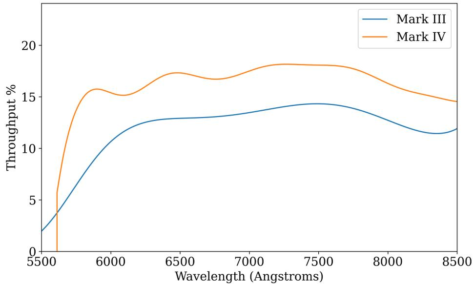
Figure 4.5: The net spectroscopic throughput of the LRIS-red spectrograph measured using PypeIt. The orange curve shows the throughput from the new Mark IV detector taken in May 2021 and the blue curve shows the throughput measure in January 2020 using the same grism (600/7500) and dichroic (560D) with the Mark III detector.
