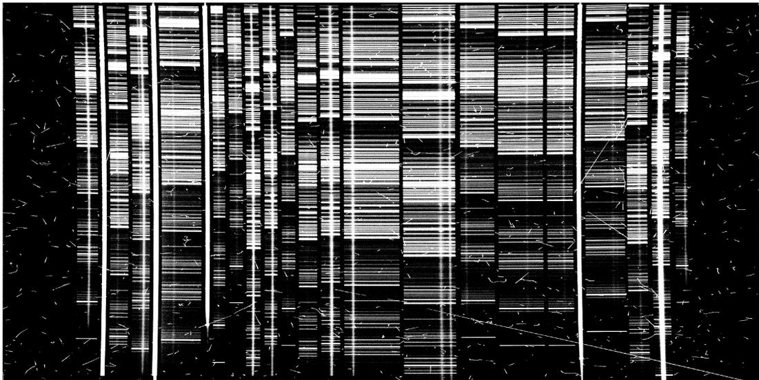
Figure 4.4: The first multi-slit spectroscopic observation obtained with the LRIS-red Mark IV. The raw file has been minimally processed: bias-subtraction, flat-fielding, and removal of the overscan regions. Note that the image contains no gap in the center as the single CCD eliminates the chip gap from LRIS red Mark III.
