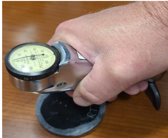
Figure 3.32. Barcol hardness impressor diagram (Left) and impressor in use (Right)
