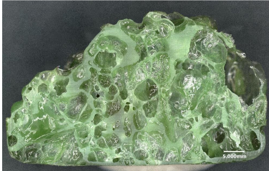
Figure 4.49. CP-2 (30% acetone diluted EA9396) cure parameter coupon section
