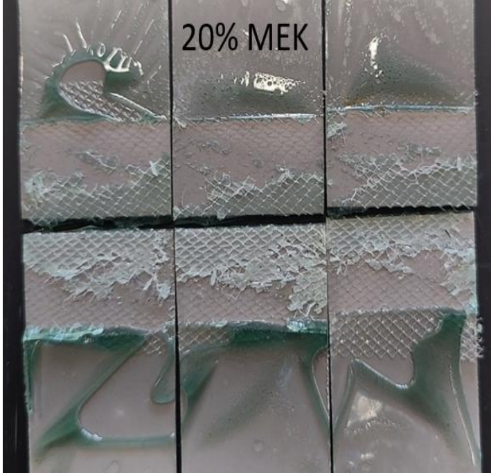
Figure B.5. LS-MEK-20 coupon failure surfaces
