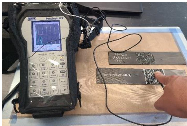
Figure 3.10. Pulse-echo ultrasonic A-scan hand inspection test set-up
