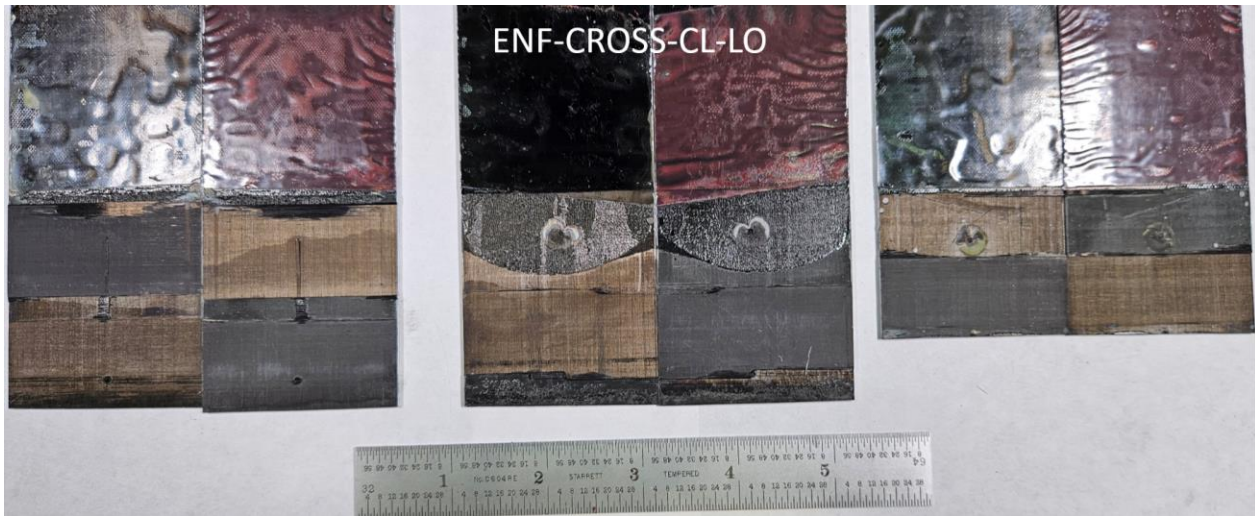
Figure C.15. ENF-CROSS-CL-LO failure surfaces
