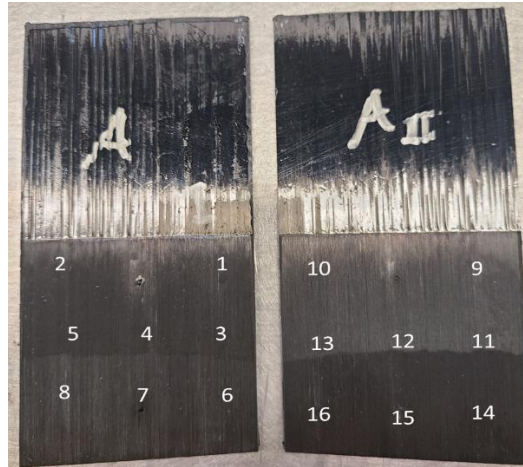
Figure 3.28. FTIR analysis locations on ENF process development coupon
