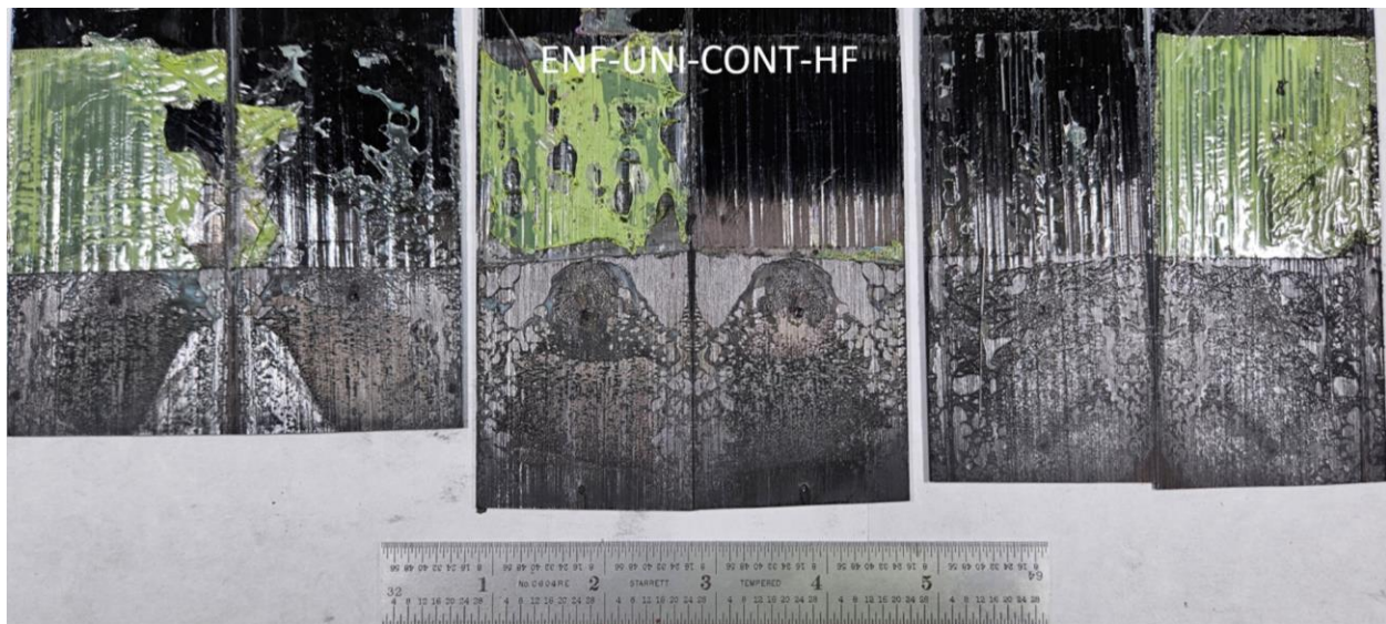
Figure C.4. ENF-UNI-CONT-HF failure surfaces
