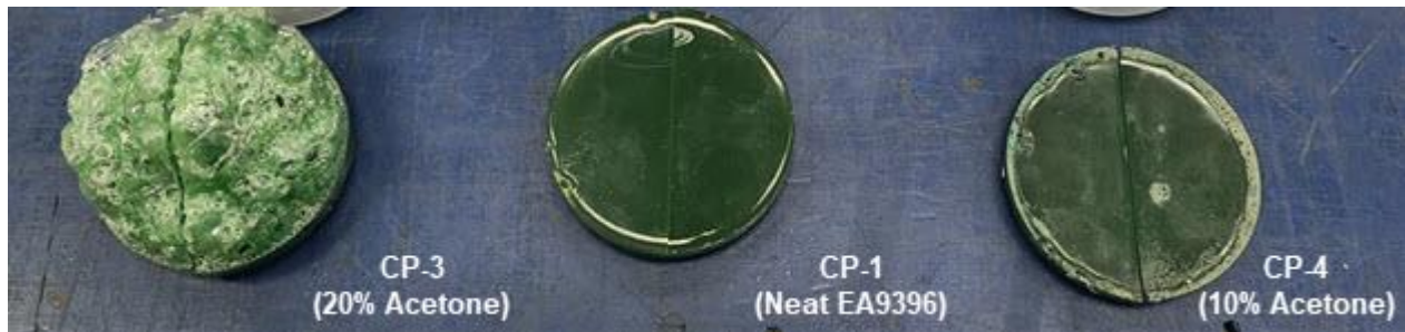
Figure 4.47. Cure parameter testing of diluted EA9396 resin puck coupons
