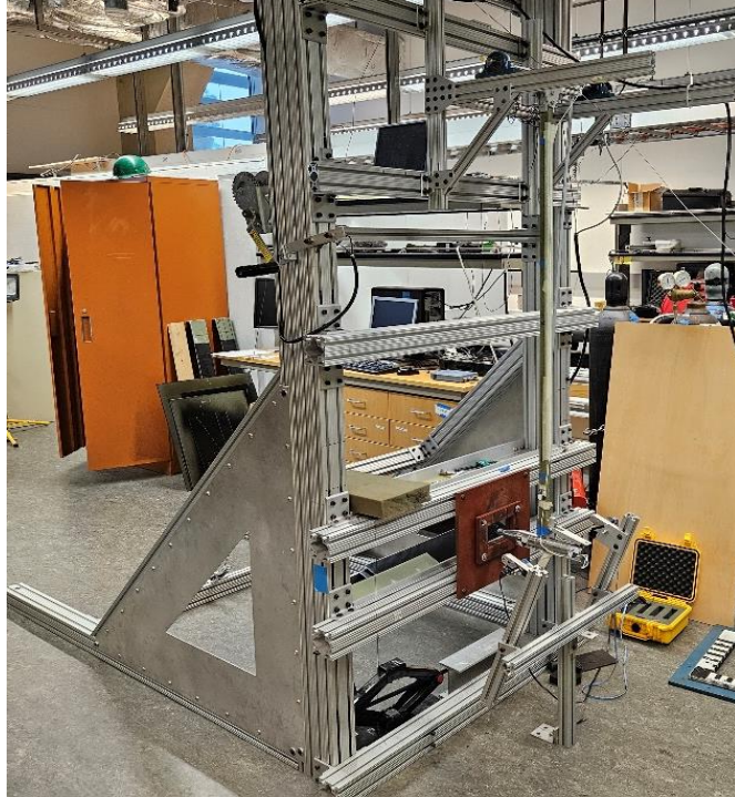
Figure 3.6. Pendulum impactor set-up
