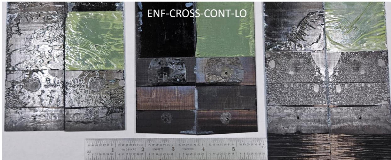
Figure C.12. ENF-CROSS-CONT-LO failure surfaces
