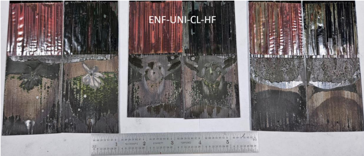
Figure C.7. ENF-UNI-CL-HF failure surfaces
