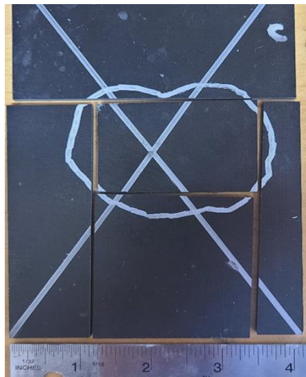
Figure 3.8. 20J impact specimen sectioned for microscopic observation
