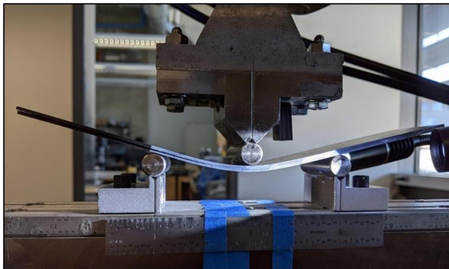
Figure 3.3. Laboratory ENF test fixture set-up and specimen during testing
