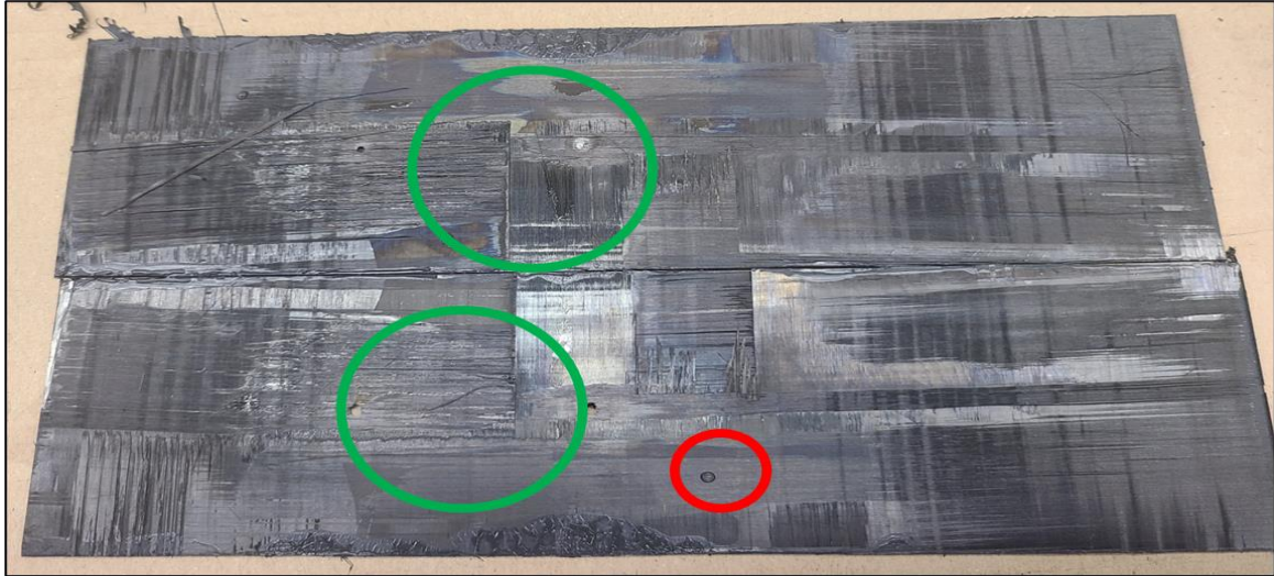
Figure 4.34. WCA readings after atmospheric plasma treatment of hydraulic fluid contaminated modified ENF coupon
