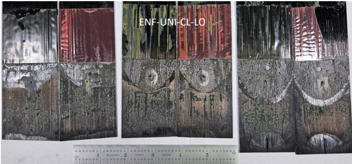
Figure C.13. ENF-UNI-CL-LO failure surfaces
