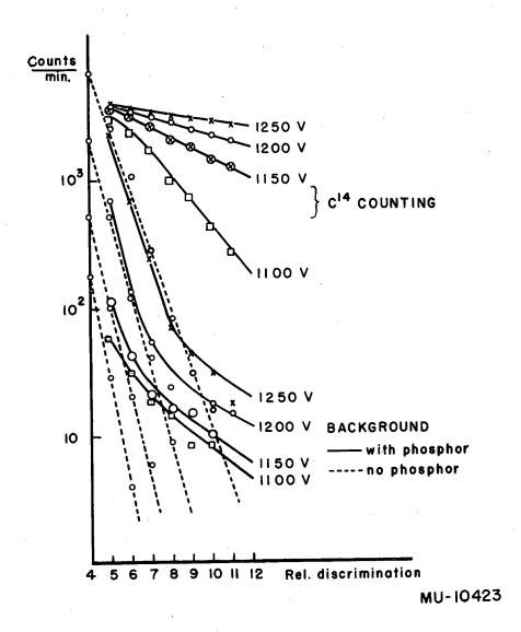
Fig. 1. Counting rate for C<sup>14</sup> sample as a function of relative discrimination of pulse height. Upper curves are for 1800-cpm. sample (G-M tube with 6 dis./ct. efficiency) and lower curves are background.
