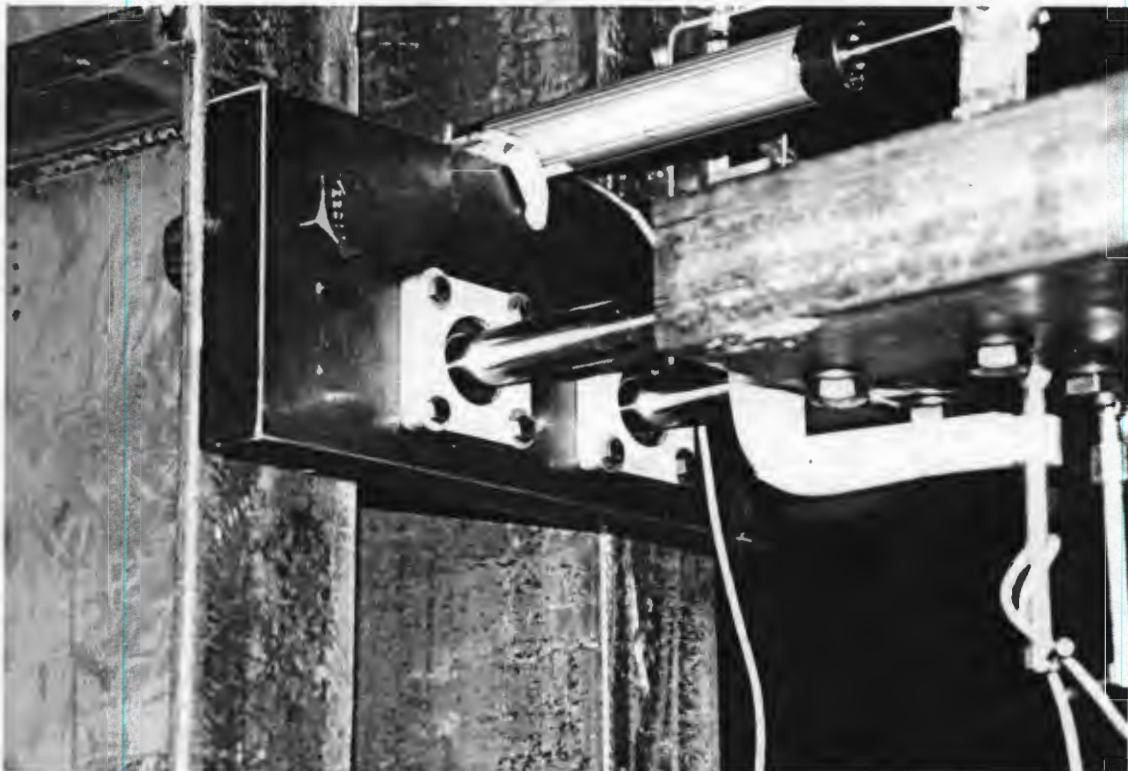
Figure 2.3. (a) Dynamic actuator, (b) Low friction linear bearings
