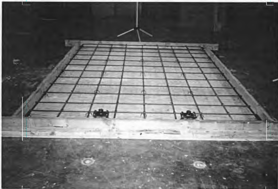
Figure 3.2. Panel formwork and reinforcement
