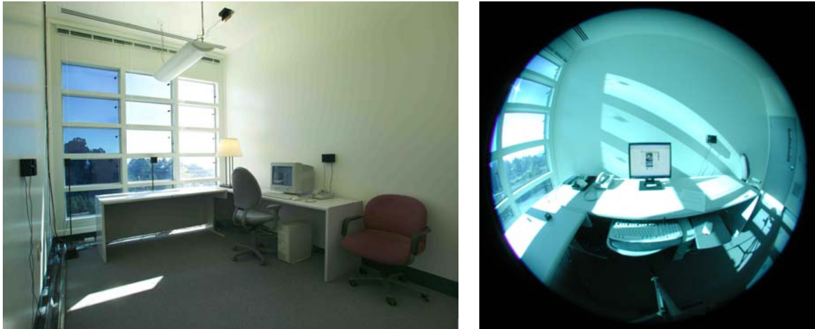
Fig. 1. Perspective (left) and fisheye (right) of test room interior. The left view shows the columns of electrochromic windows at three different levels of transmittance: 5%, 30%, and 60%. The right view shows the window at 5%. The rooms were not furnished with a task desk lamp (shown in left figure) at the time of the tests.
