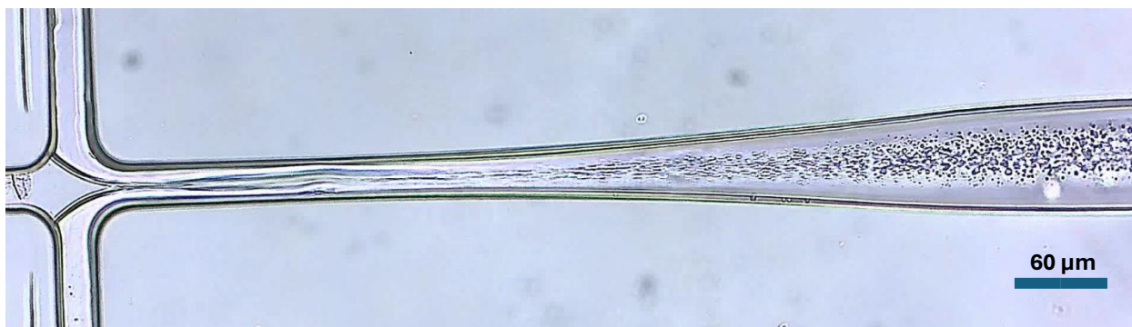
Figure 8: Schematic of the microfluidic flow-focusing channel structure used to disperse bulk homogeneous coacervates into relative supernatant. All the channels at the junction are 30 \mu\text{m} and the outlet is expanding to 80 \mu\text{m} gradually. Homogeneous bulk coacervate phase enters the junction from left and is pinched and focused by a much faster sheath flow of supernatant stream entering the junction from the channels at the top and bottom.
