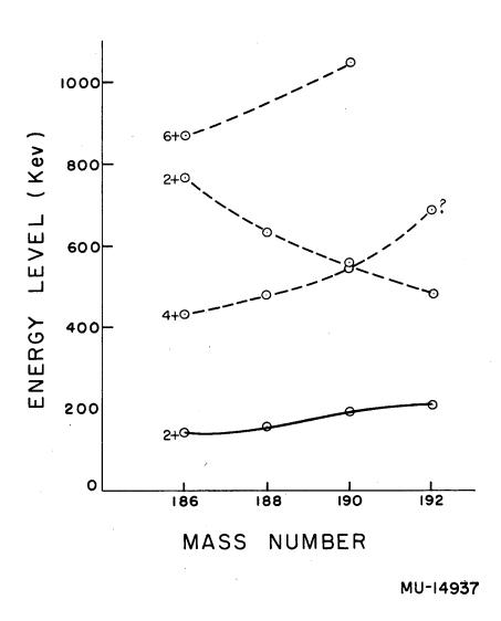
Fig. 3. Correlation diagram of energy levels of even-mass osmium nuclei.
