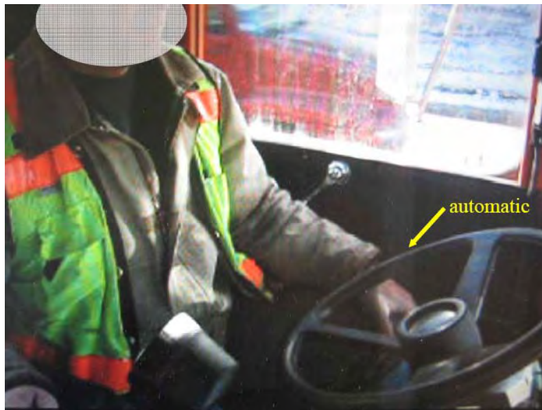
Figure 13. 18 Operator using automated steering control along I-80 guardrail
