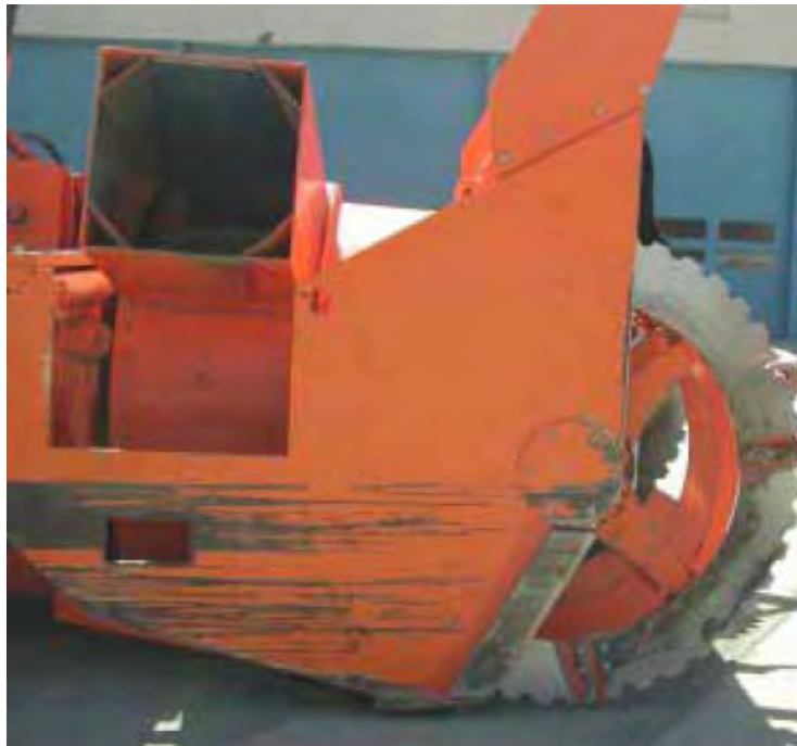
Figure 1. 2 Example of a blower head with scratch mark
