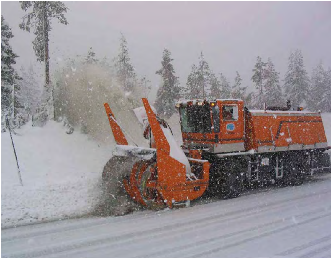
Figure 1. 4 Rotary Snowblower in Operation near Donner Summit.
