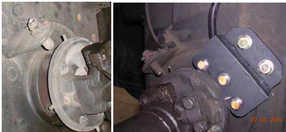
Figure 6. 5 Speed sensor (left: old; right: improved)
