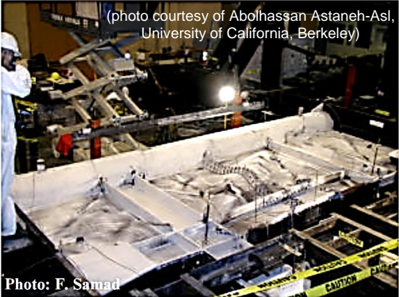
Specimen 1 at 3.3% Drift
