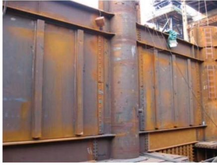
(a) Buckling restrained SPSW Type I: channel stiffener with a gap between end of stiffeners to the boundary beams by Lee et al. (2010)
