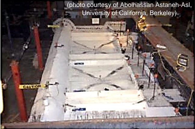
Specimen 2 at 2.2% Drift
