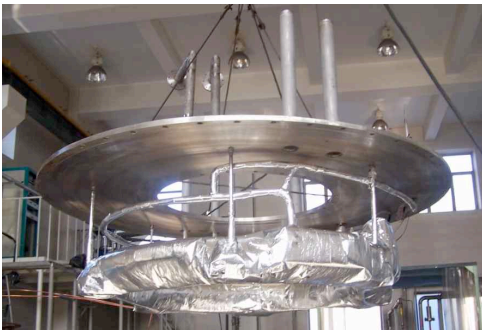
Figure 7: Installation of the Large coil in its Cryostat.
