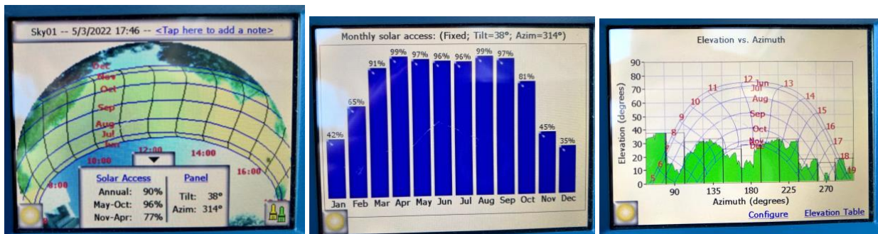
Figure 8. Screen shots from the Solmetric SunEye 210 showing the solar access yearly projection charts and shade coverage.
